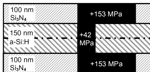
Fig. 4. Schematic diagram showing the stress status of stacked layers.
