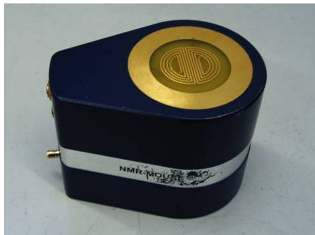
Fig. 5. The handheld single bar magnet MOUSE. The field strength at the surface is approximately 0.46 T, equating to a proton resonance frequency of 19 MHz. The strength of the alternating field produced by the B_1 coil for 100 W of RF power is 1.5 mT and the typical B_1 pulse duration is 4 \mu s [4, 9].
