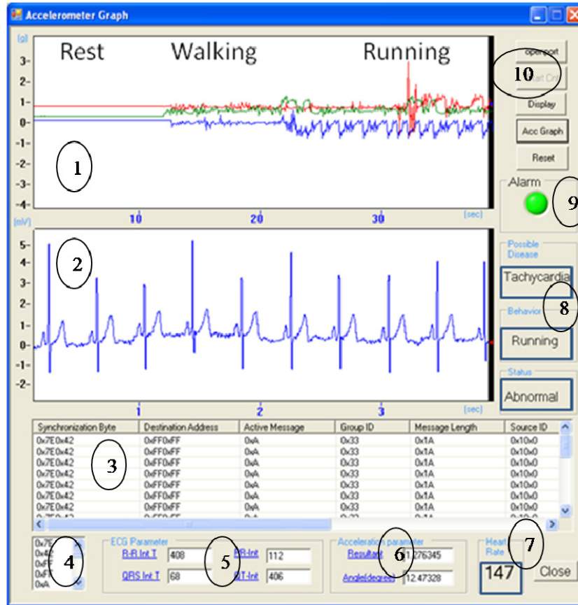
Fig. 10. An ECG and Accelerometer interface with abnormal status on Server: R-R interval= 408 ms, QRS width = 68 ms, QT interval= 406 ms, PR interval = 112 ms, Resultant = 1.276345, Angle (degree) = 12.47328 and HR = 147. ECG data is taken by MIT-BIH arrhythmia database and accelerometer data is received by sensor node attached to the human body.
