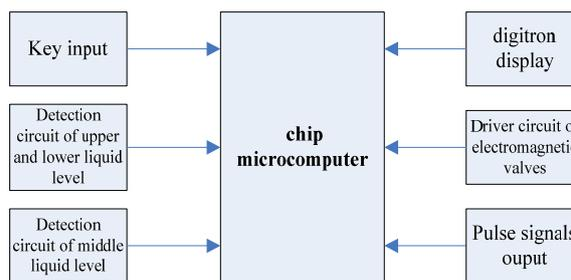
Fig. 2. Systematic diagram of electric-controlling system.
