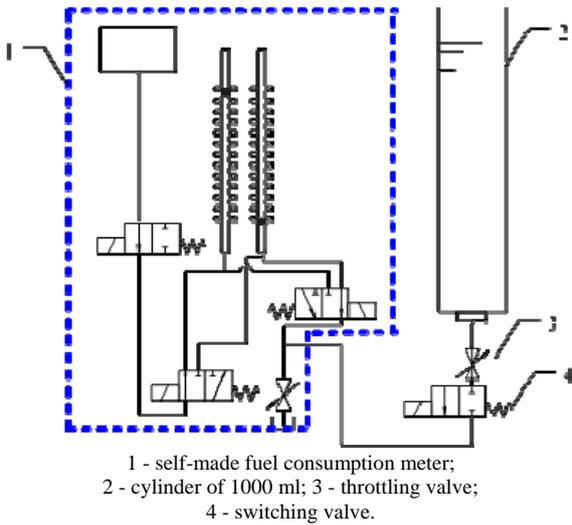
Fig. 10. Chart of precision calibration bench.
