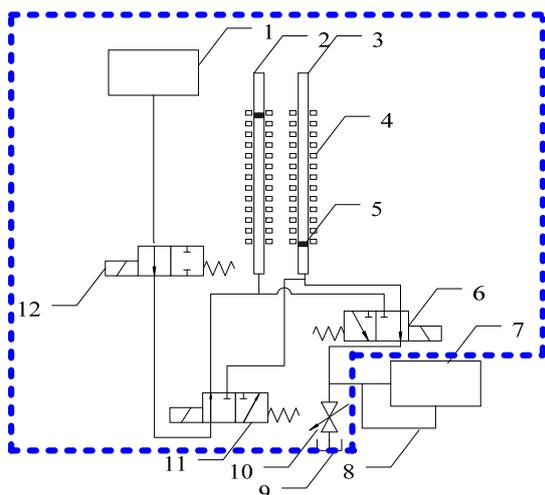
1 - external fuel tank; 2 - Alkali burette; 3 - Alkali burette; 4 - photoelectric sensors; 5 - Float (light-proof); 6 - reversing valve; 7 - engine; 8 - engine fuel return pipe; 9 - tank; 10 - throttling valve; 11 - reversing valve; 12 - switch valve.
