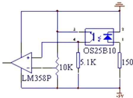
Fig. 4. Circuit of photoelectric sensors.
