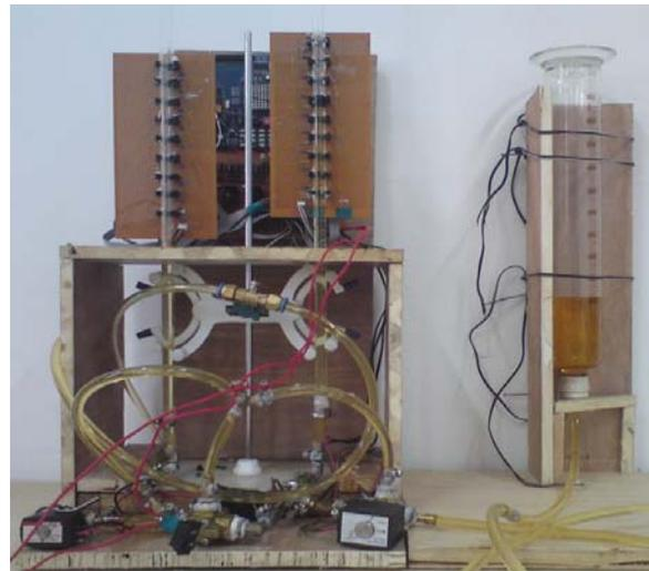
Fig. 11. Self-made fuel consumption meter and calibration device.
