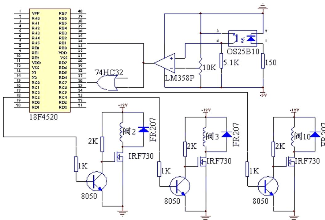
Fig. 6. Design of the control system’s circuit.
