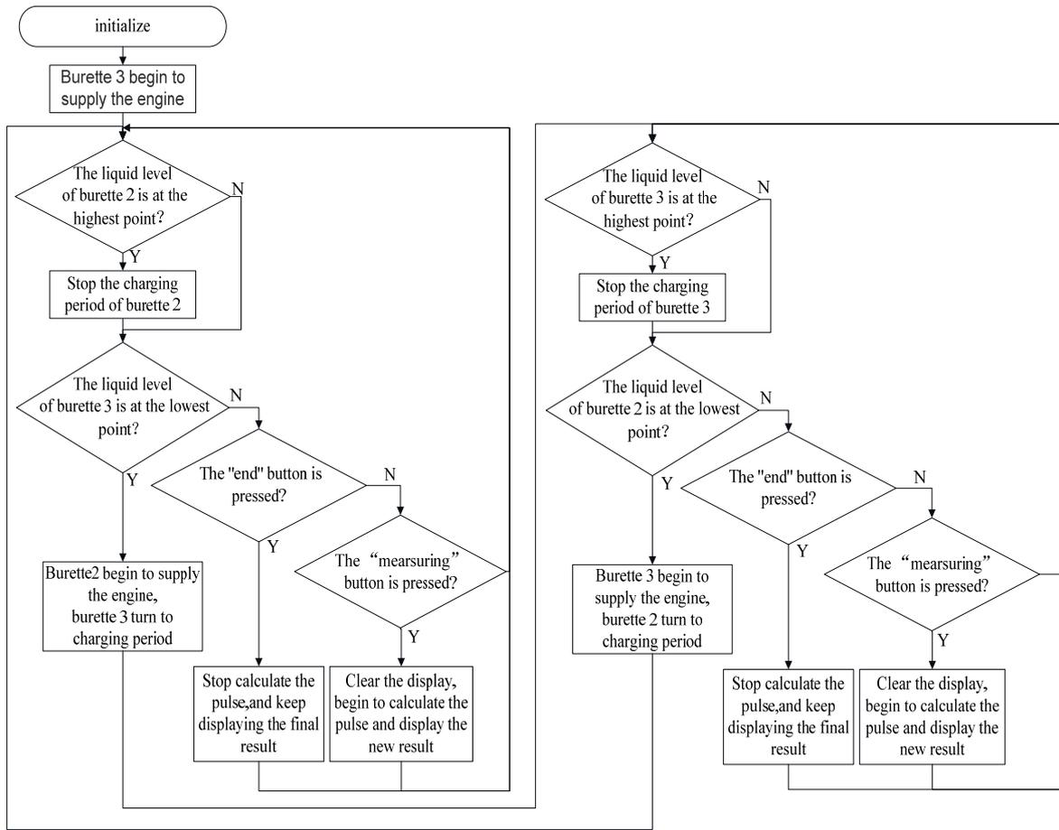
Fig. 9. Flowchart of measuring.
