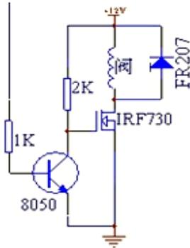
Fig. 3. The controlling circuit of electromagnetic valves.
