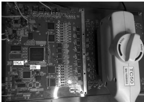
Fig. 6. Prototype board of medical ultrasound scanner.
