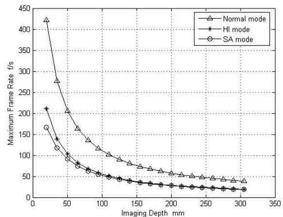
Fig. 7. Maximum frame rate under 120 scanlines.
