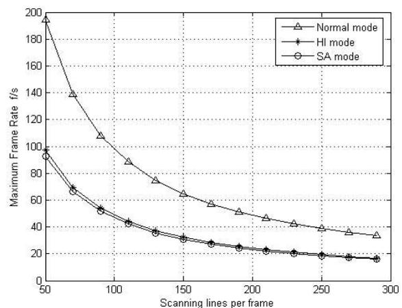
Fig. 8. Maximum frame rate under the imaging depth of 150 mm.
