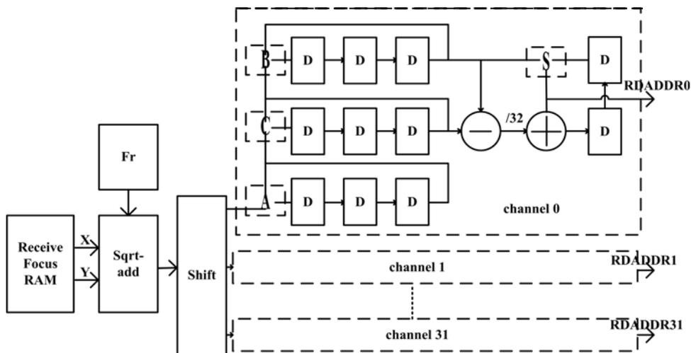
Fig. 4. Structure of reading addresses generator.
