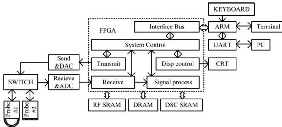
Fig. 2. Functional block of ultrasound imaging system.
