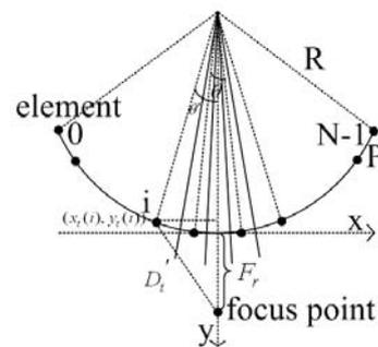
Fig. 1. Mathematical model of time-of-flight calculation.
