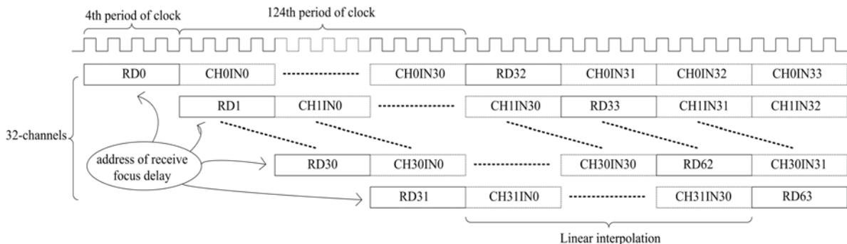
Fig. 5. Timing relationship of the generated addresses.
