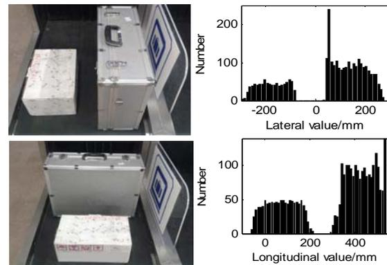
Fig. 8. Distributions of laser data in horizontal and vertical directions.
