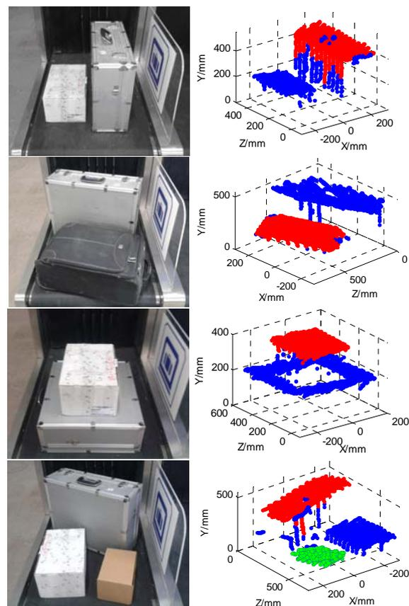
Fig. 9. Clustering segmentation for laser point cloud.
