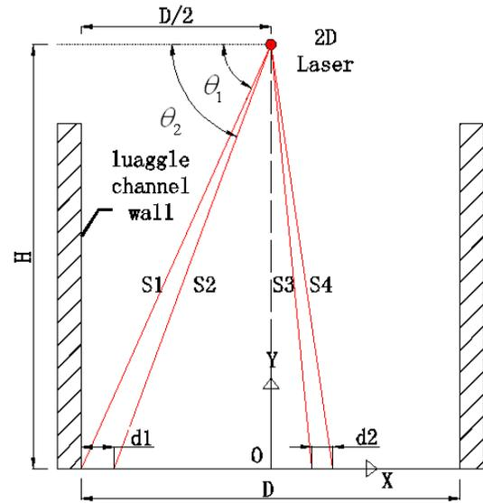
Fig. 3. The error analysis of single laser in X direction.
