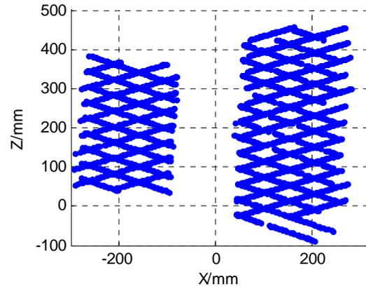
Fig. 5. Laser point cloud of multiple pieces of luggage.
