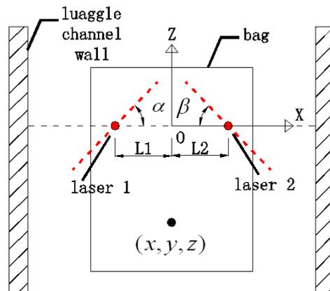
Fig. 2. Installation of dual lasers over top view.
