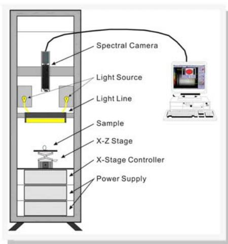
Fig. 1. Hyperspectral imaging system.
