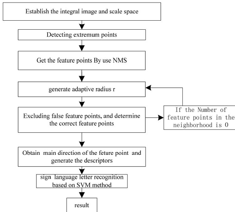
Fig. 2. The improved algorithm flow chart.
