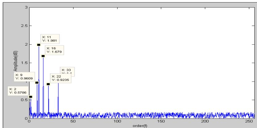
**Fig. 6.** The order cepstrum of gear misalignment.
