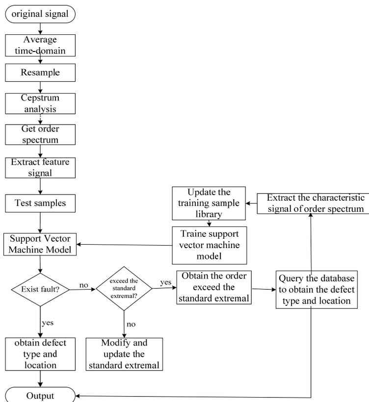
Fig. 1. The flow chart of quality detection.
