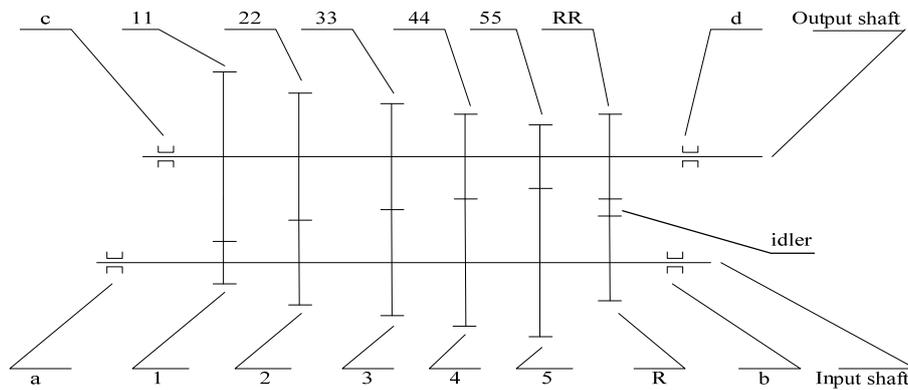
Fig. 3. The internal structure diagram of the transmission.
