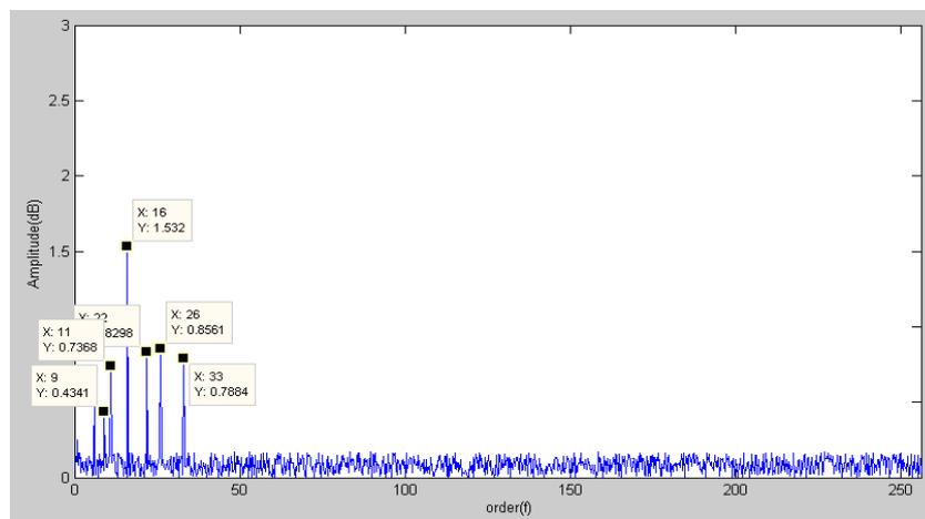
**Fig. 7.** The order cepstrum of surface machining error of gear.
