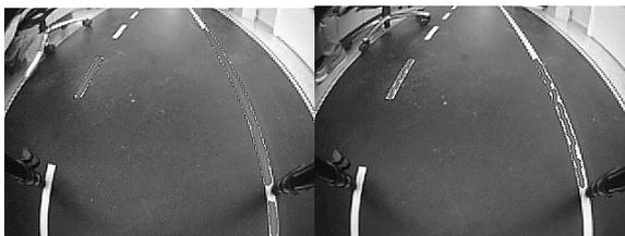
Fig. 4. Hough-lines and sorted points along the Hough-lines.
