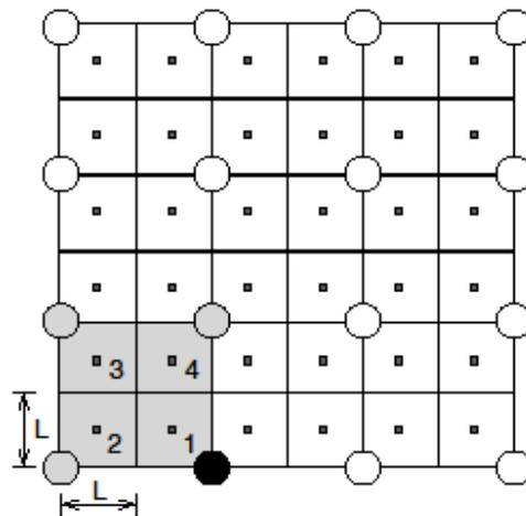
Fig. 1. Layout of sensors (circles) and fingerprint points (dots) over an area of interest.
