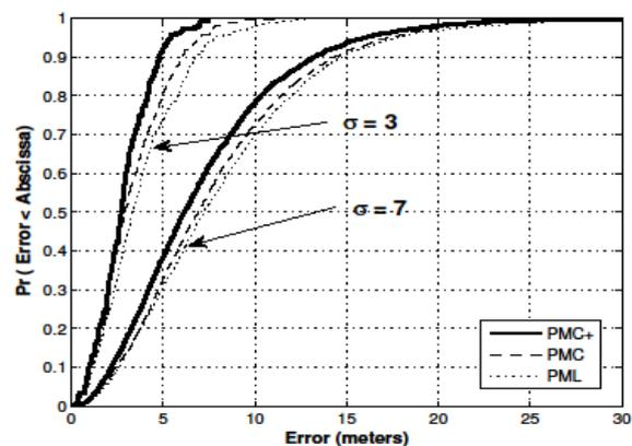
Fig. 2. Estimation error comparison of PMC+, PMC and PML, Square Region Simulation.
