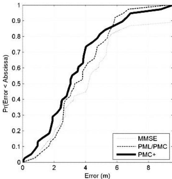
Fig. 9. Estimation error comparison of PMC+, PML and PML, Kingsbury Hall Measurement Campaign.
