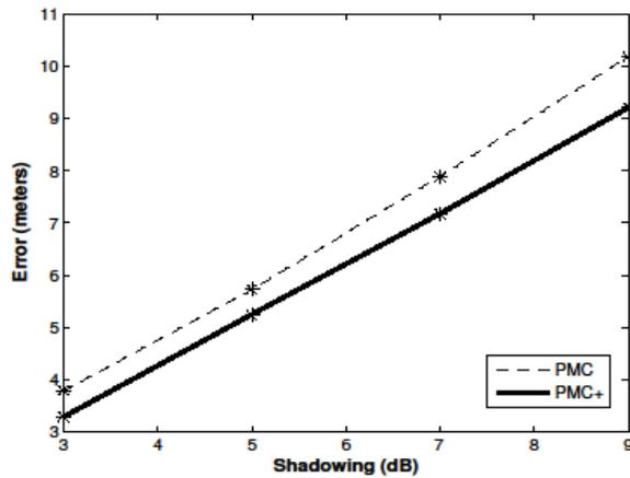
Fig. 3. Mean error of PMC+ and PMC for different values of shadowing power,  $\sigma$  (dB), Square Region Simulation.
