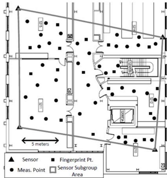
Fig. 4. Map of Kingsbury Hall, South Wing, Second Floor, including sensors, fingerprint points and measurement points.
