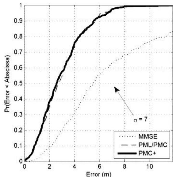
Fig. 7. Estimation error comparison of PMC+, PML and PML, Kingsbury Hall Simulation,  $\sigma = 7$ .
