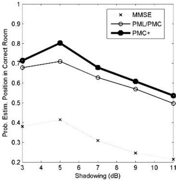
**Fig. 8.** Probability of Correct Room Estimation for PMC+, PML/PMC and MMSE for different values of  $\sigma$  (dB).
