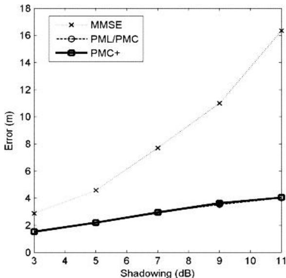
Fig. 5. Mean error of PMC+ and PMC for different values of shadowing power,  $\sigma$  (dB), Kingsbury Hall Simulation.
