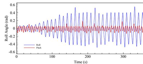
**Fig. 6.** Roll and pitch motions in parametric roll resonance.
