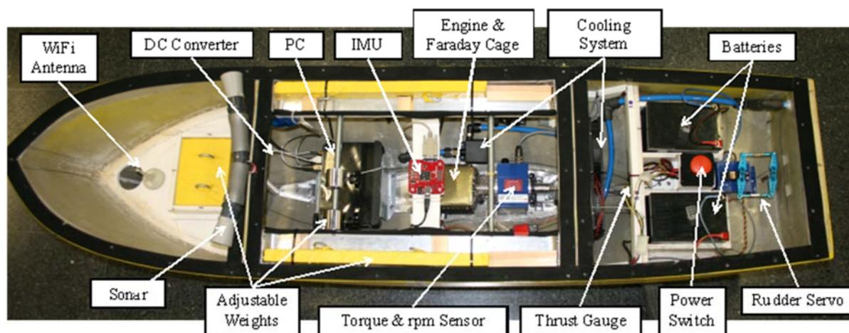
Fig. 1. Ship scale model overview.
