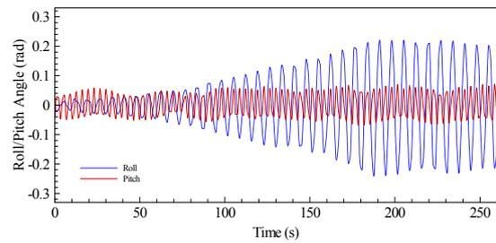
Fig. 9. Roll and pitch motions in parametric roll resonance. Proposed model.
