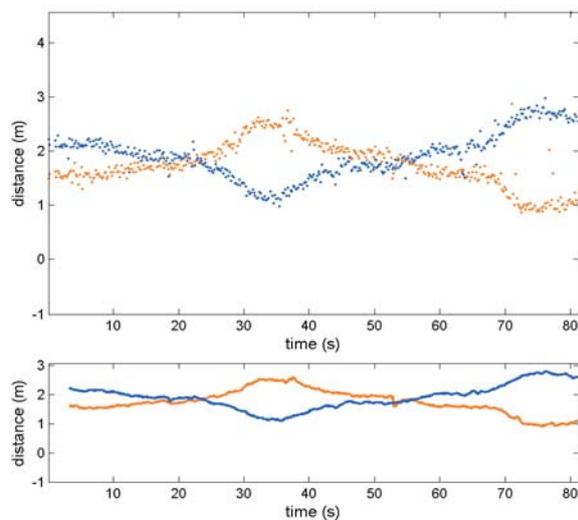
**Fig. 4.** Raw (top) and filtered (bottom) measurements from the left (red) and right (blue) sonars.
