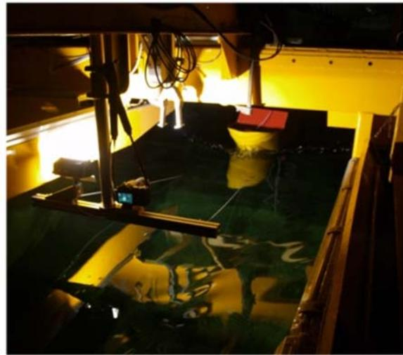
**Fig. 5.** Conventional carriage-towed model during testing.
