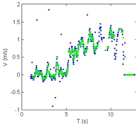
**Fig. 2.** Raw (blue dots) and filtered (green dots) velocity values obtained by differentiation of the LRF signals.
