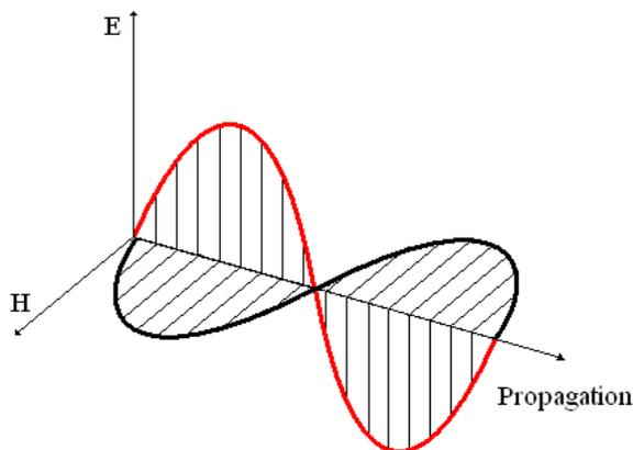
Fig. 1. Scheme of electromagnetic wave propagation.
