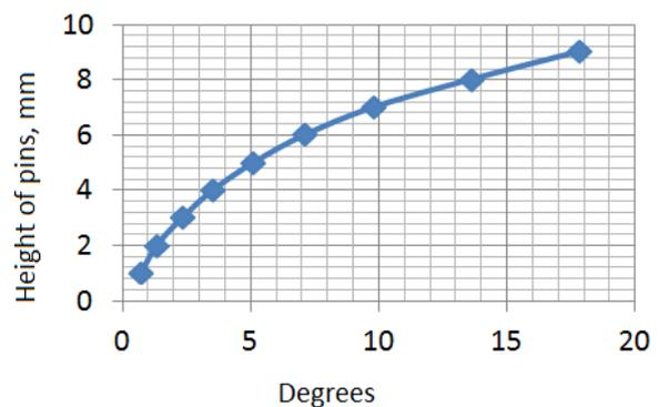
Fig. 9. Dependence of the phase shift by increasing the height of pins.
