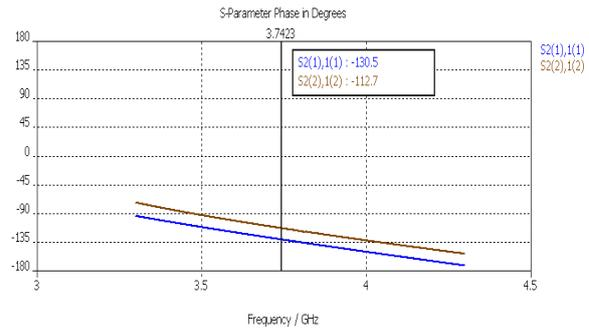
Fig. 8. The phase delay between vertically and horizontally polarized signal.
