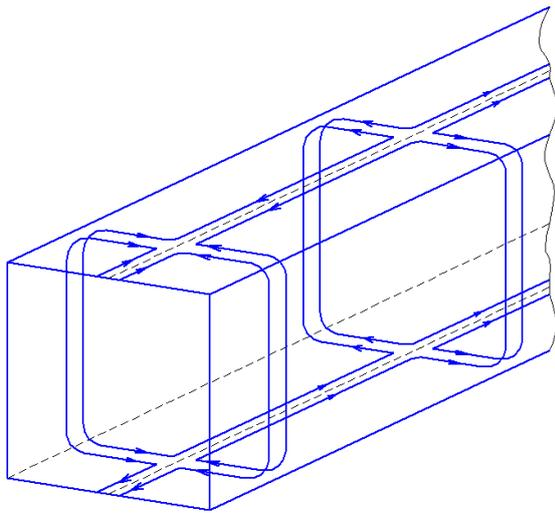
Fig. 2. Distribution of currents on the walls of the polarizer.
