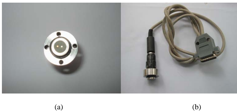
Fig. 1. Top view of the sensor showing the electrodes supported by the dental acrylic (a); sensor with cable and connector (b).
