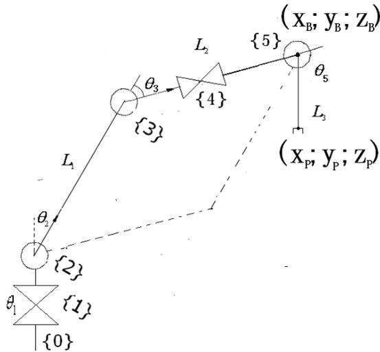
Fig. 2. Coordinate corresponding to attitude of end position of weld.
