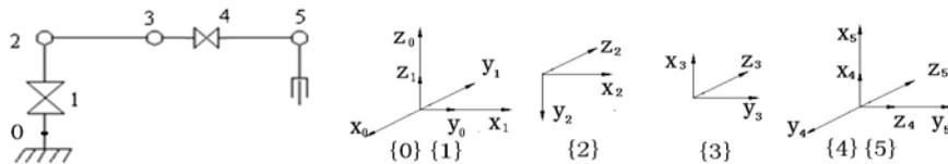
Fig. 1. Six Cartesian coordinates for welding robots of three-arm and five-degree freedom plus large scope of traversing.
