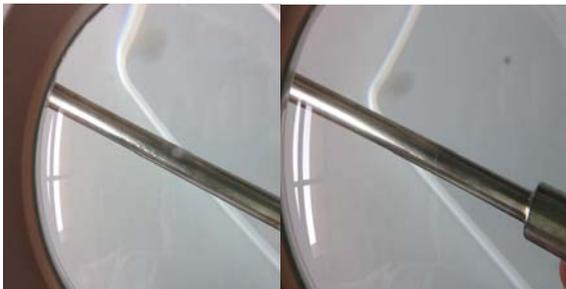
Fig. 11. The breakage of the stem.
