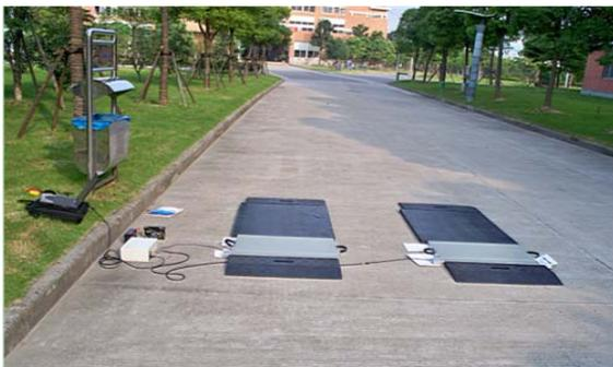
**Fig. 8.** Experimental site of vehicle weigh-in-motion.
