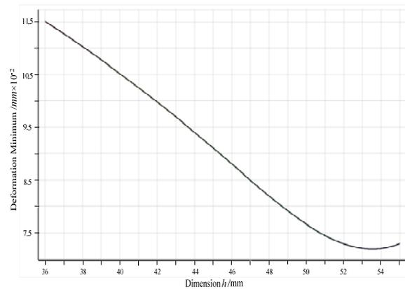
Fig. 6. The width-deformation relationship curve.
