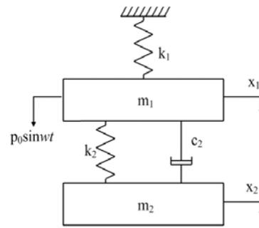
Fig. 2. Physical model of the vibration absorption system.
