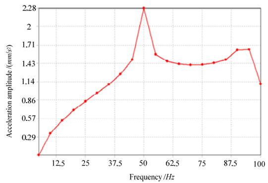
Fig. 8 (c). Comparison of the damping effect in acceleration amplitude: after the optimization.
