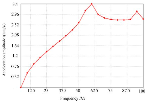
Fig. 8 (b). Comparison of the damping effect in acceleration amplitude: before the optimization.
