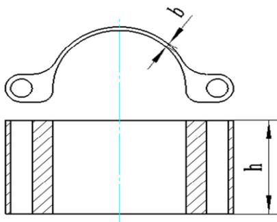
Fig. 4. Geometry of the C-spring in DVA.
