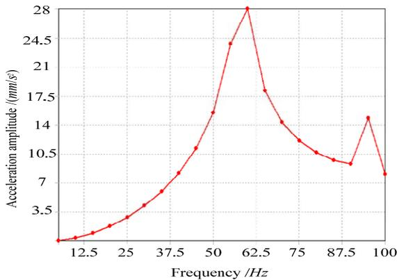
Fig. 8 (a). Comparison of the damping effect in acceleration amplitude: without the DVA.
