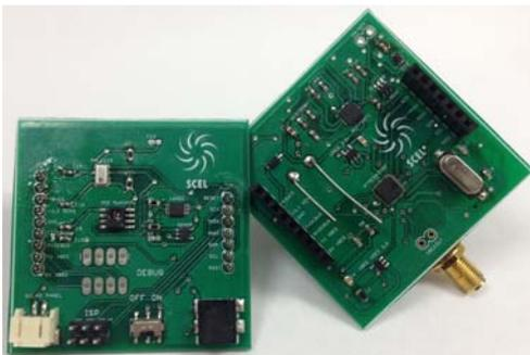
**Fig. 1.** Primary components of current sensor node: main board and sensor board.
