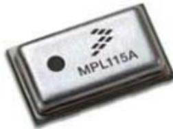
Fig. 4. MPL115A2 barometer.
