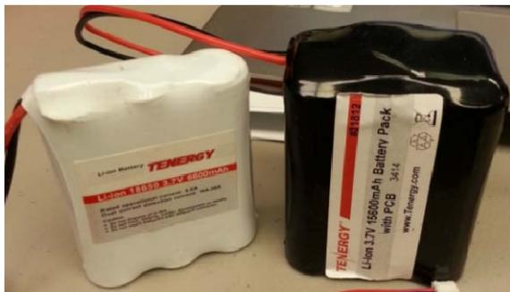
Fig. 5. Battery for previous sensor module (left), and battery for current sensor module (right).
