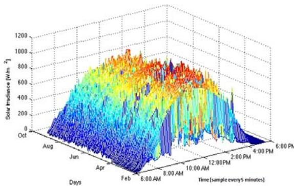
**Fig. 11.** Solar irradiance (SI) data before filter with moving average filter, and standard normalization.
