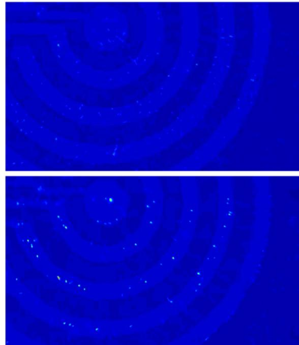
**Fig. 6.** *E. coli* expressing GFP (green) and resuspended in water from the Charles River in Cambridge, MA was captured on the Fluid-Screen cell sorter. Images were taken before (top) and 30 seconds after (bottom) application of the electric field. Magnification, 10X.
