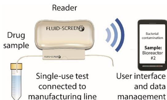
**Fig. 8.** Design of the optimized Fluid-Screen integrated bacterial detector unit, including the cell sorter presented here and a proprietary bacterial identification component. A sterile disposable chip inserts into a handheld Bluetooth-enabled portable reader. Microfluidic pumps process the fluid sample. After 30 minutes (assuming flow of 100 mL), results are transmitted to a smartphone or a central database.
