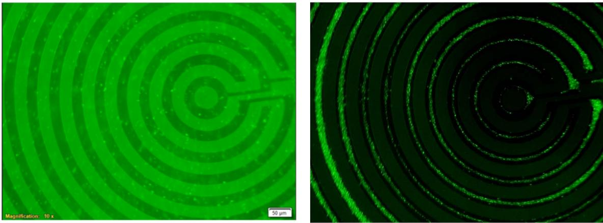
**Fig. 2.** *E. faecalis* expressing GFP (green) and captured on the Fluid-Screen cell sorter at 10x magnification. Images were taken before (top) and 30 seconds after (bottom) application of the electric field.
