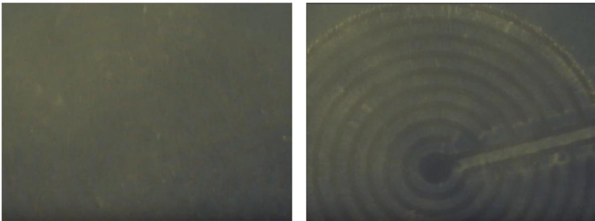
**Fig. 3.** *B. subtilis* expressing mCherry (red) and captured on the Fluid-Screen cell sorter at 10x magnification. Images were taken before (top) and 60 seconds after (bottom) application of the electric field. Notice both the collection of bacteria on the electrode and the structured alignment of the rod-shaped organisms after electric field application.
