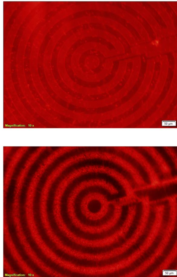
**Fig. 1.** *E. coli* expressing mCherry (red) and captured on the Fluid-Screen cell sorter at 10x magnification. Images were taken before (top) and 30 seconds after (bottom) application of the electric field. Note the uniform cell distribution before field application, and both the rearrangement and the increase in cell number 30 seconds after application.
