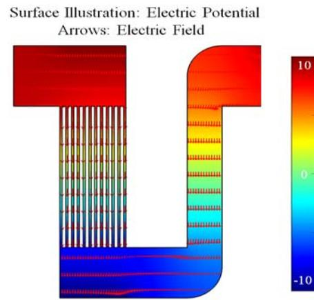
Fig. 4. Electric potential surface plot and corresponding generated uniform electric field inside the channel, indicated with red arrows.
