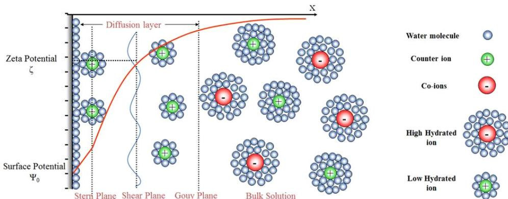
**Fig. 2.** Electric double layer formation; the whole ions in bulk solution are highly surrounded by water molecules, so the bulk solution is electrically neutral. However, due to the electrochemical effect at surface, the ions are low hydrated (by water molecules) near the solid-wall/electrolyte interface. So, a thin layer charged by counter-ions, at interface between the solid wall and electrolyte.
