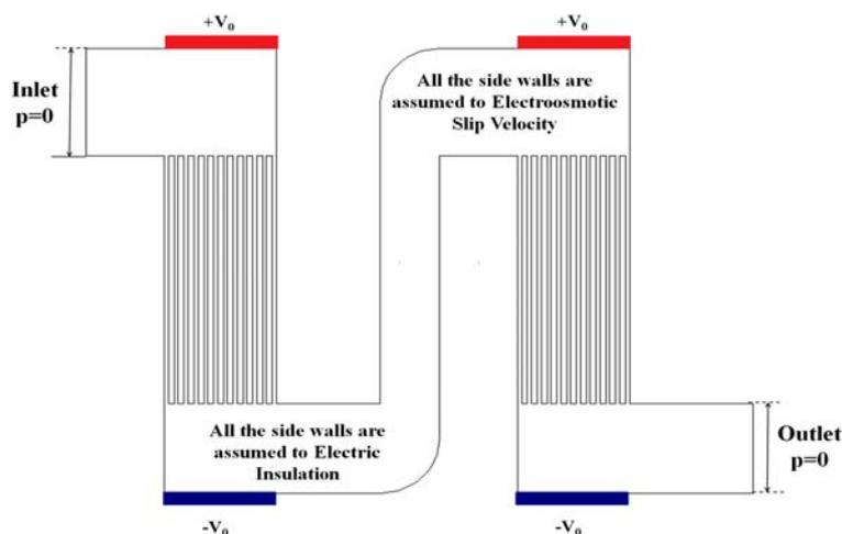
**Fig. 3.** Micropump boundary conditions for both Fluid flow and electric field.
