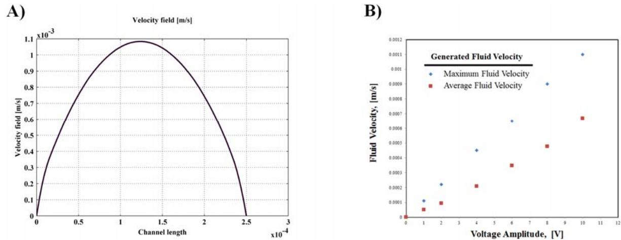
Fig. 6. Velocity results; (A) velocity profile at outlet and (B) voltage variation effect on pumping velocity.
