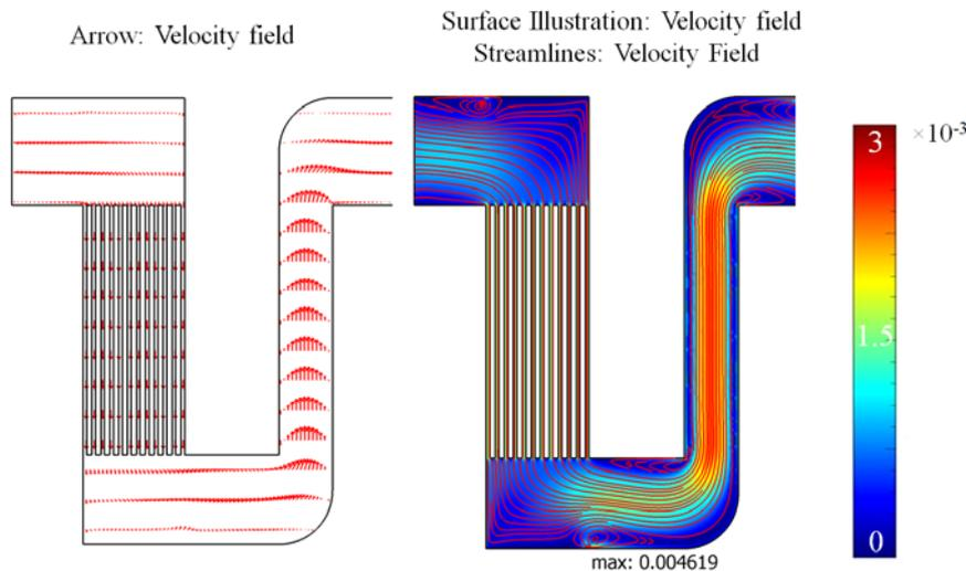
Fig. 5. Velocity field inside the microchannel; including arrows, streamlines and surface plot.
