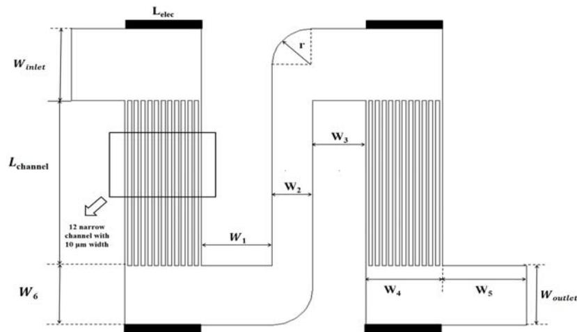
**Fig. 1.** Two-dimensional Schematic view of microchannel and narrow microchannels, four microelectrodes are placed in the top and down of microchannel for pumping process.
