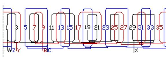
(b) 22 pole number stator winding with 36 slots
