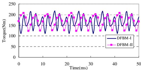
**Fig. 9.** Torque versus time of two DFBMs.
