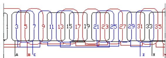
(a) 8 pole number stator winding with 36 slots
