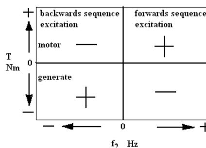
Fig. 4. Power flow in the control (secondary) winding.
