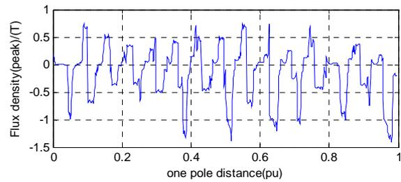
Fig. 8 (a). Air-gap flux density waveform and its harmonics of DFBM-II: Flux density for outer air-gap.
