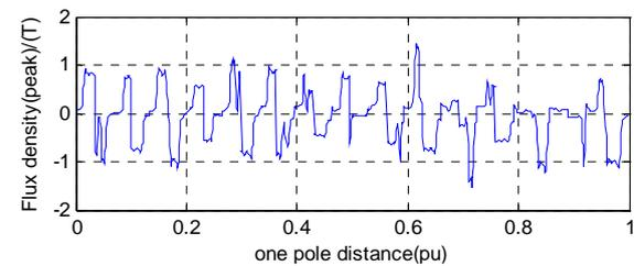
Fig. 8 (c). Air-gap flux density waveform and its harmonics of DFBM-II: Flux density for inner air-gap.
