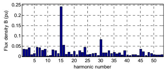
Fig. 8 (b). Air-gap flux density waveform and its harmonics of DFBM-II: Harmonics for outer air-gap.
