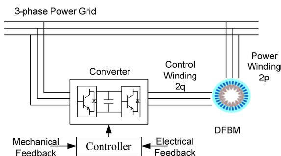
Fig. 2. Schematic diagram of a DFBM system.
