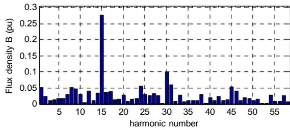
**Fig. 8 (d).** Air-gap flux density waveform and its harmonics of DFBM-II: Harmonics for inner air-gap
