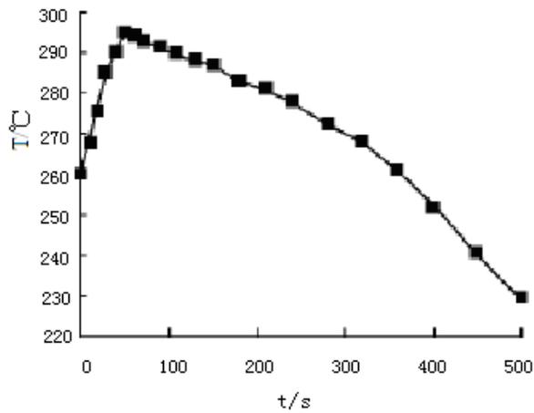
Fig. 3. The cooling temperature curve of brake shoe on the surface.
