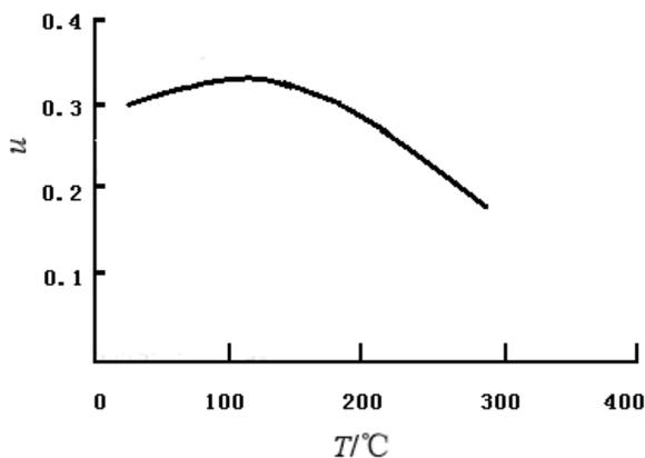
Fig. 4. Relation between the brake shoe friction coefficient and the surface temperature.
