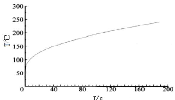
Fig. 2. The temperature curve of the brake shoe on the surface.
