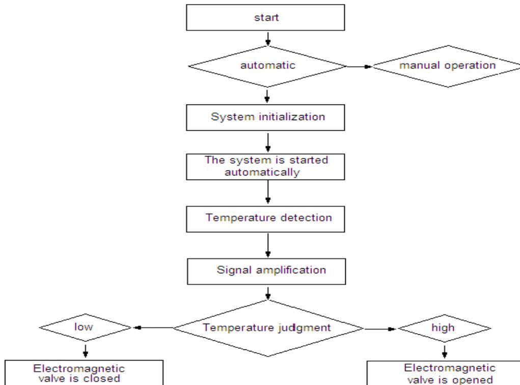
Fig. 1. The system work procedure.
