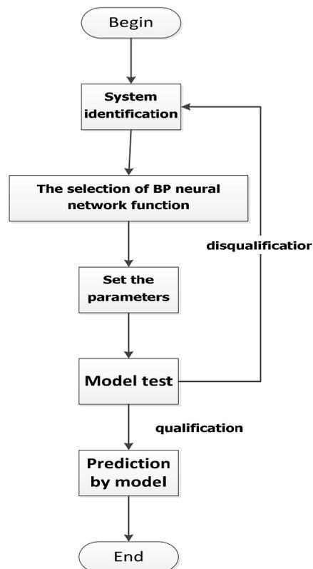
Fig. 4. The flow chart of BP neural network.
