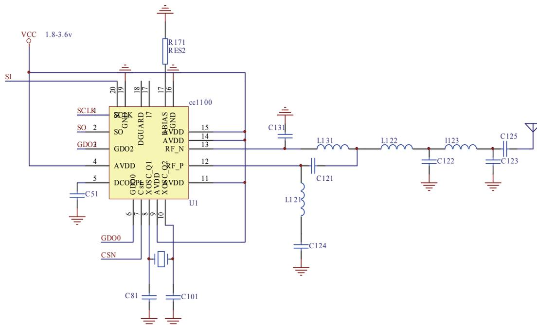
Fig. 4. CC1100 Application Circuit.
