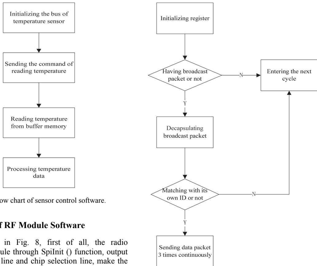
Fig. 7. Flow chart of sensor control software.
