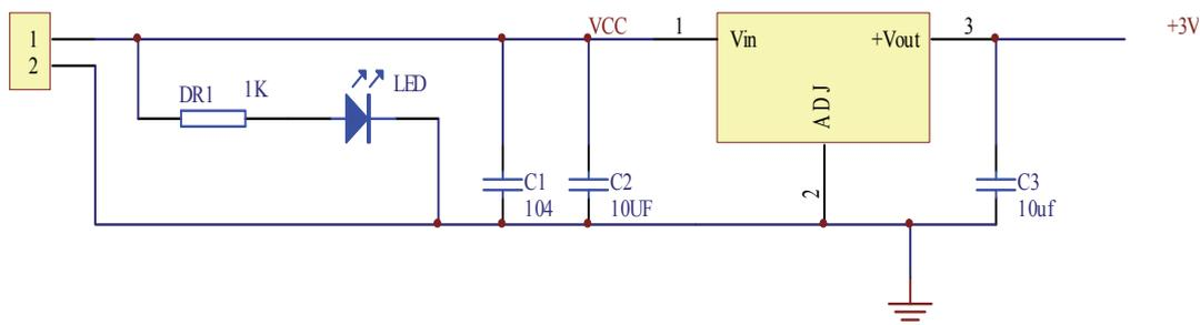
**Fig. 5.** ASM117 stable voltage circuit.
