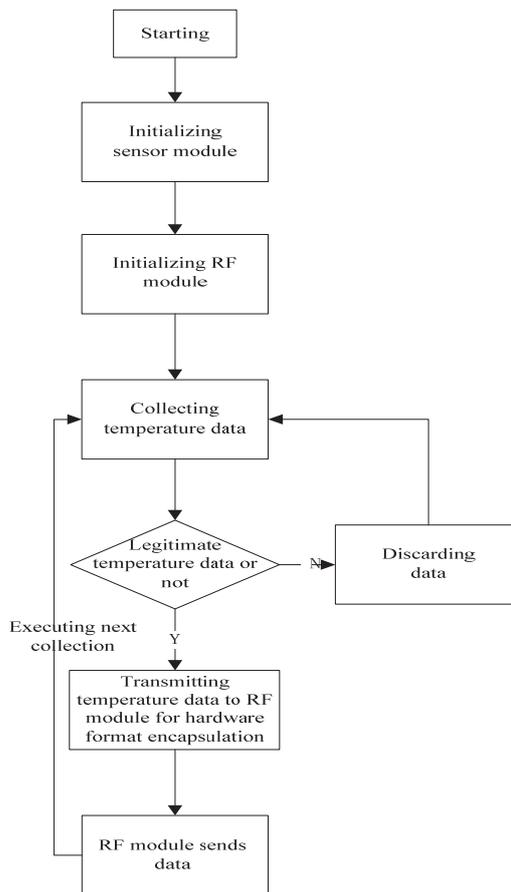
Fig. 9. Overall operational process.
