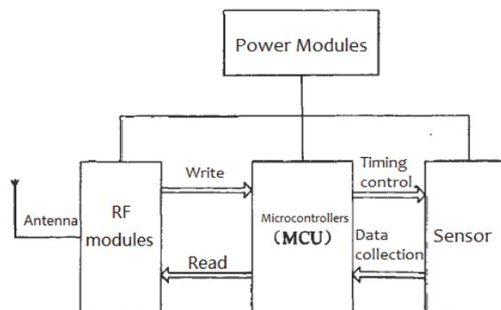
Fig. 3. Sensor label structure.
