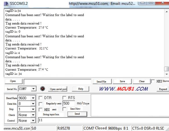
**Fig. 11.** Broadcast command of reader to read three tags.
