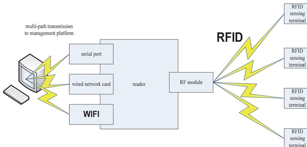
Fig. 1. System structure.
