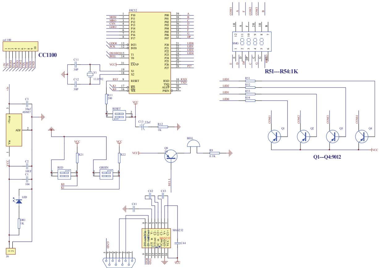
Fig. 6. The principle diagram of electronic label control module.
