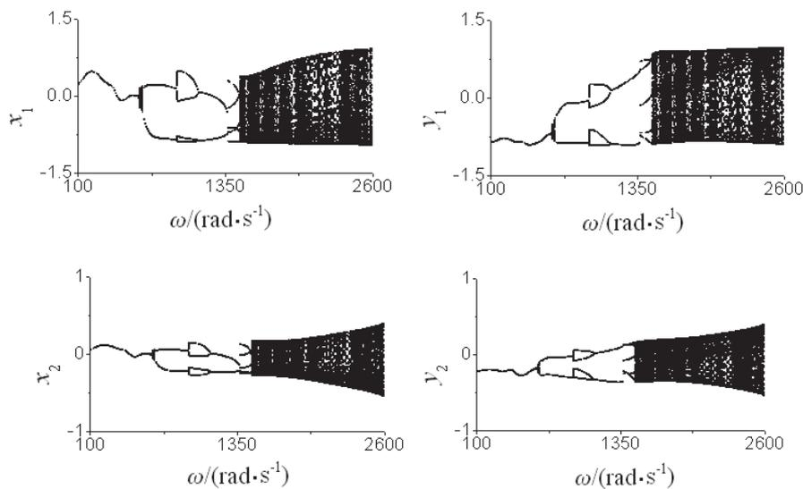
Fig. 2. The bifurcation diagrams of rotor response with  $\omega$ .
