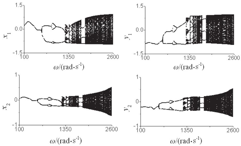
**Fig. 4 (b).** The bifurcation diagrams of rotor response with  $\omega$  at different crack depth  $a=0.7$ .
