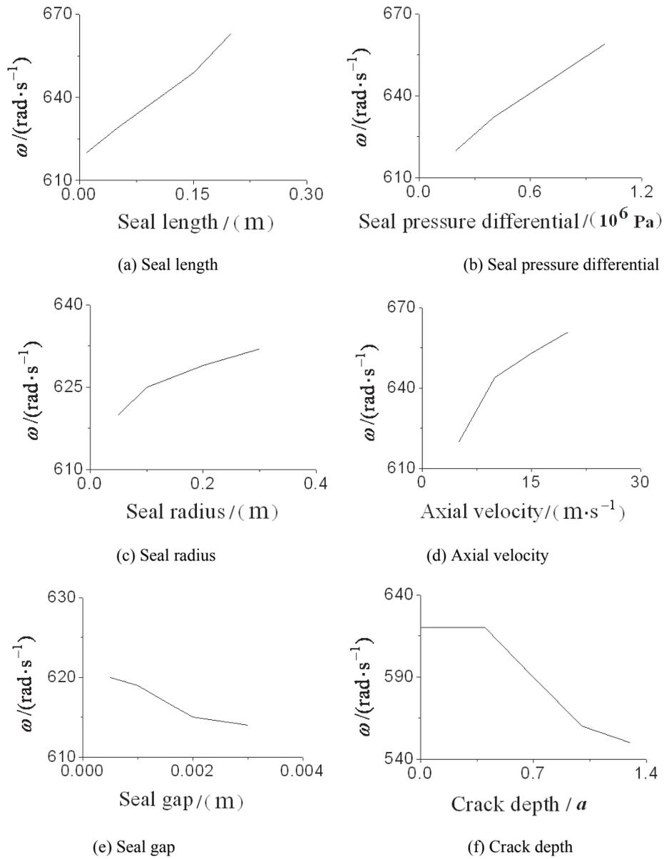
Fig. 3. Effects of parameters on critical unstable rotating speed.
