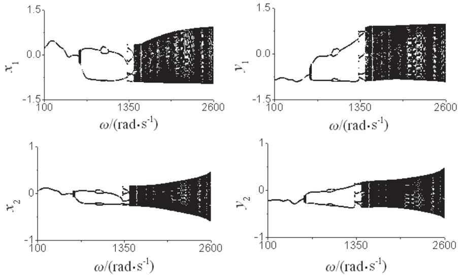
Fig. 4 (a). The bifurcation diagrams of rotor response with  $\omega$  at different crack depth  $a=0.4$ .
