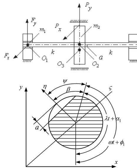
Fig. 1. Models of rotor-bearing-seal coupling system and section of crack.
