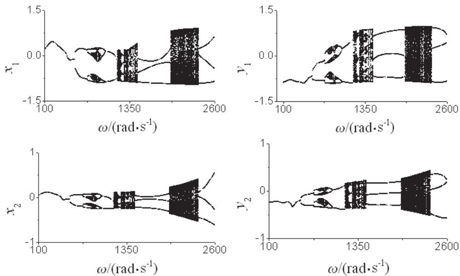
**Fig. 4 (d).** The bifurcation diagrams of rotor response with  $\omega$  at different crack depth  $a=1.3$ .
