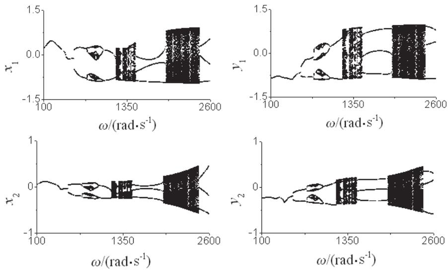
**Fig. 4 (c).** The bifurcation diagrams of rotor response with  $\omega$  at different crack depth  $a=1.0$ .
