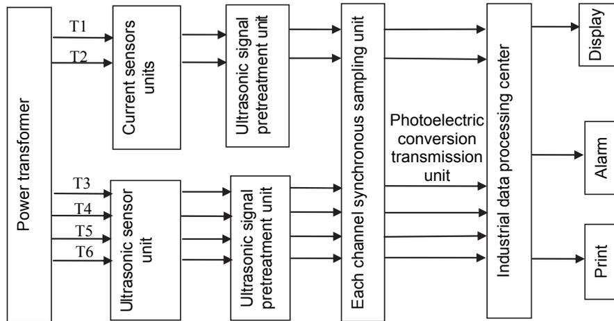
Fig. 1. The structure diagram of the electro-acoustic joint monitoring system.
