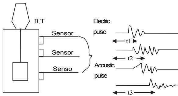
Fig. 2. The working principle of ultrasonic detection system.
