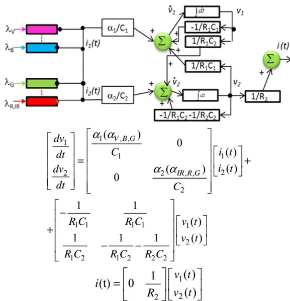
Fig. 3. Block diagram and linear state equations.
