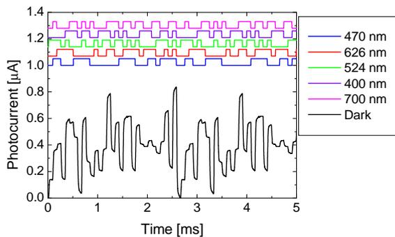
**Fig. 11.** Multiplexed output (Dark) with random data in channels 400 nm, 470 nm, 524 nm, 626 nm, 700 nm.
