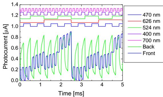
**Fig. 10.** Multiplexed signal with channels 400 nm, 470 nm, 524 nm, 626 nm, 700 nm, with back or front ultra-violet steady state illumination.
