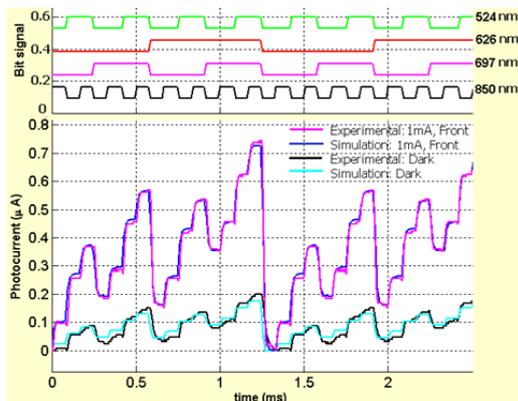
Fig. 4. Simulation example of the MUX signal with and without front  $\lambda=390$  nm irradiation.
