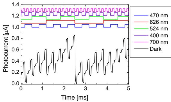
**Fig. 9.** Multiplexed signal with channels 400 nm, 470 nm, 524 nm, 626 nm, 700 nm, without ultra-violet steady state illumination.
