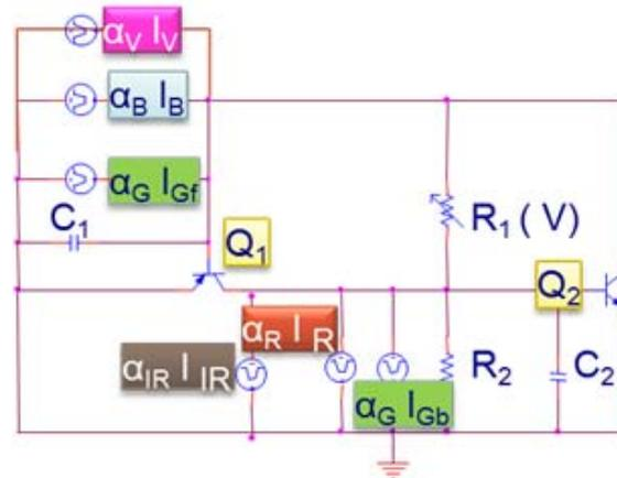
Fig. 2. ac equivalent circuit of the pi'npin photodiode.
