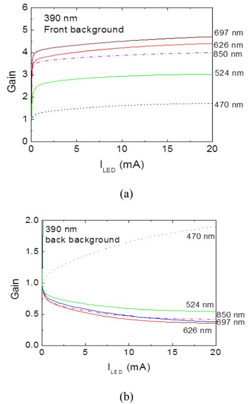
Fig. 7. a) Front and b) back optical gain at  $\lambda=390$  nm irradiation and different input wavelengths.
