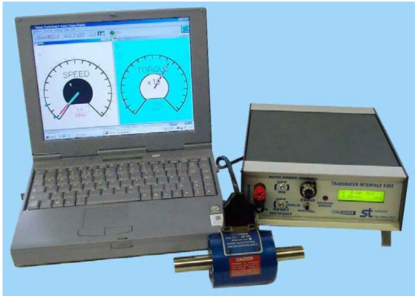
A portable PC, a Sensor Technology TORQSENSE™ torque transducer, and an E-series instrument.
