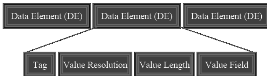
Fig. 1. DICOM Data Element Structure.
