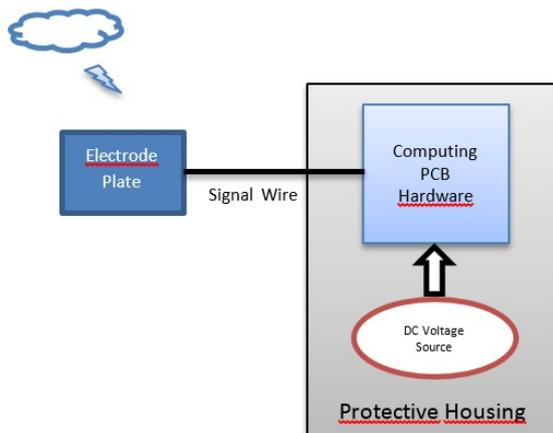
Fig. 4. Operational Scheme of Charge transfer Ice sensing.
