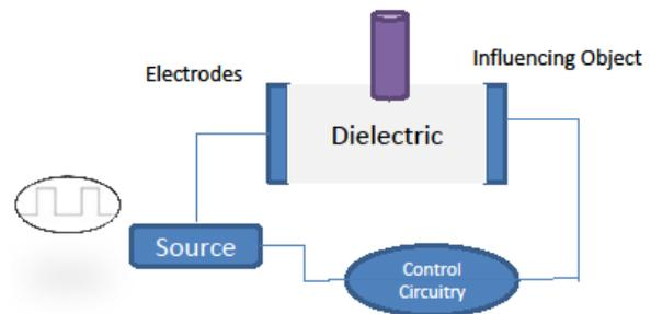
Fig. 2. Ice Detection by Mutual Capacitance (Broad Scope).
