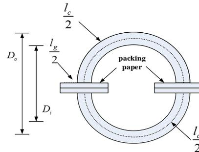
Fig. 7. Magnetic core with packing paper.
