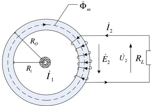
Fig. 1. Principle diagram of energy harvesting device.
