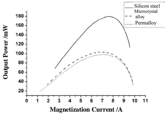
Fig. 9. Typical power output curves of magnetic cores in 3 materials.
