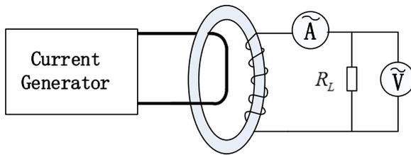
Fig. 3. Diagram of experimental circuit of output power.
