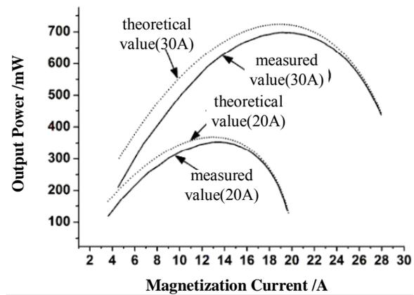
Fig. 5. Measured value and theoretical value (I1=20 A, I1=30 A).
