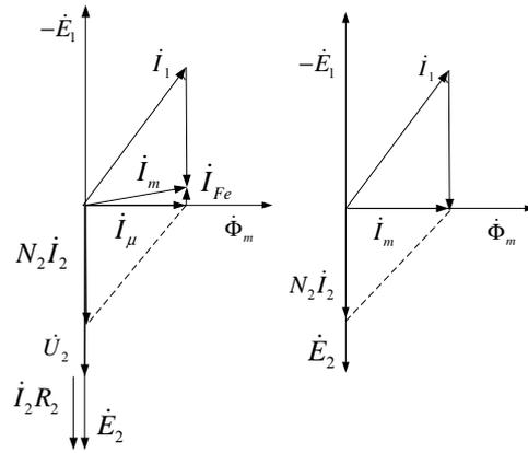
Fig. 2. Phasor diagram and simplified phasor diagram.
