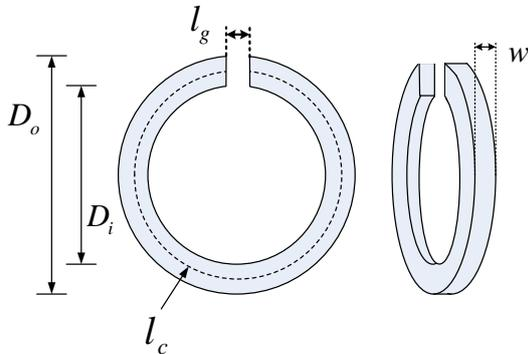
Fig. 6. Magnetic core with air gap.
