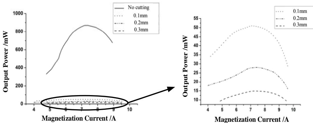
Fig. 8. Output power curves of magnetic core with packing paper.
