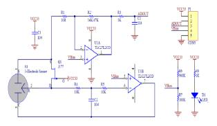
Fig. 4. Measurement circuit of NO<sub>2</sub> and HCHO.
