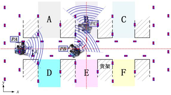
Fig. 3. Schematic diagram of tag number read by the forklift when it is moving.
