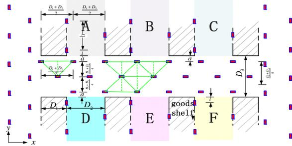
Fig. 2. Schematic diagram of arrangement of passageway signs reference tags.
