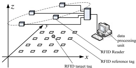
Fig. 1. Schematic diagram of RSSI positioning algorithm.
