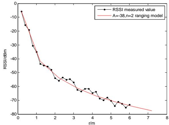
Fig. 5. Comparison of RSSI value computed by model and the actual measured value.
