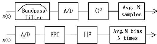
Fig. 1. The detection process implementation in time domain and frequency domain.
