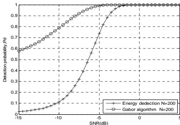
Fig. 3. The detection probability of the sample frequency taking 200.
