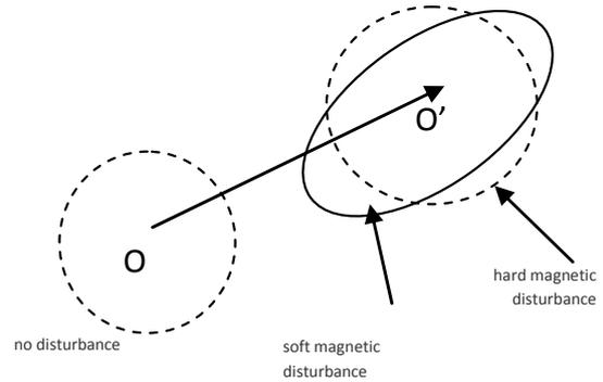
Fig. 1. 2D magnetic field trajectory measured by strap-down magnetometer.
