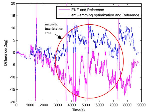
**Fig. 5.** Difference between EKF and anti-jamming.
