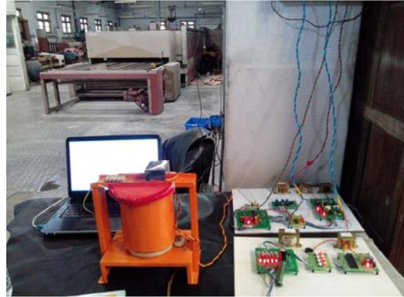
Fig. 4. Online temperature monitoring module.
