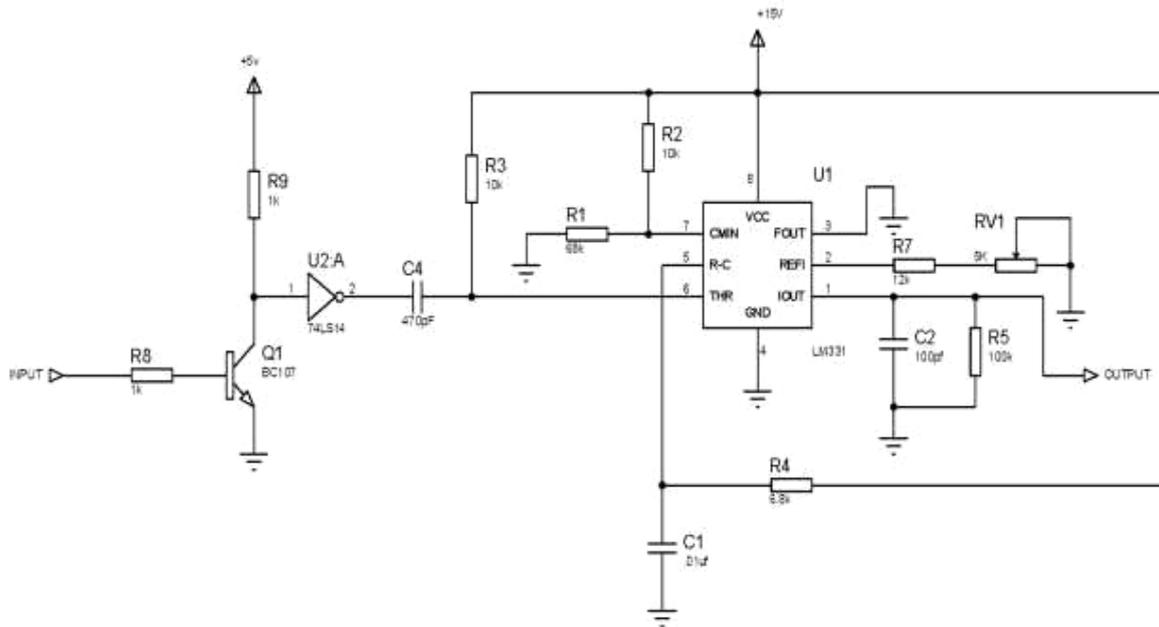
Fig. 3 (b). Receiver circuit of measuring system.
