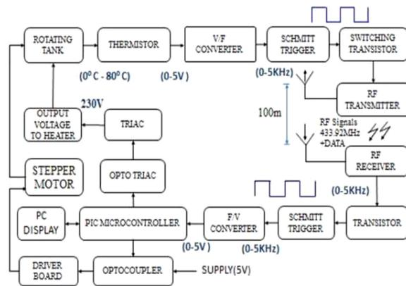
Fig. 2. Block diagram of wireless module for the measurement of temperature in a rotating drum.
