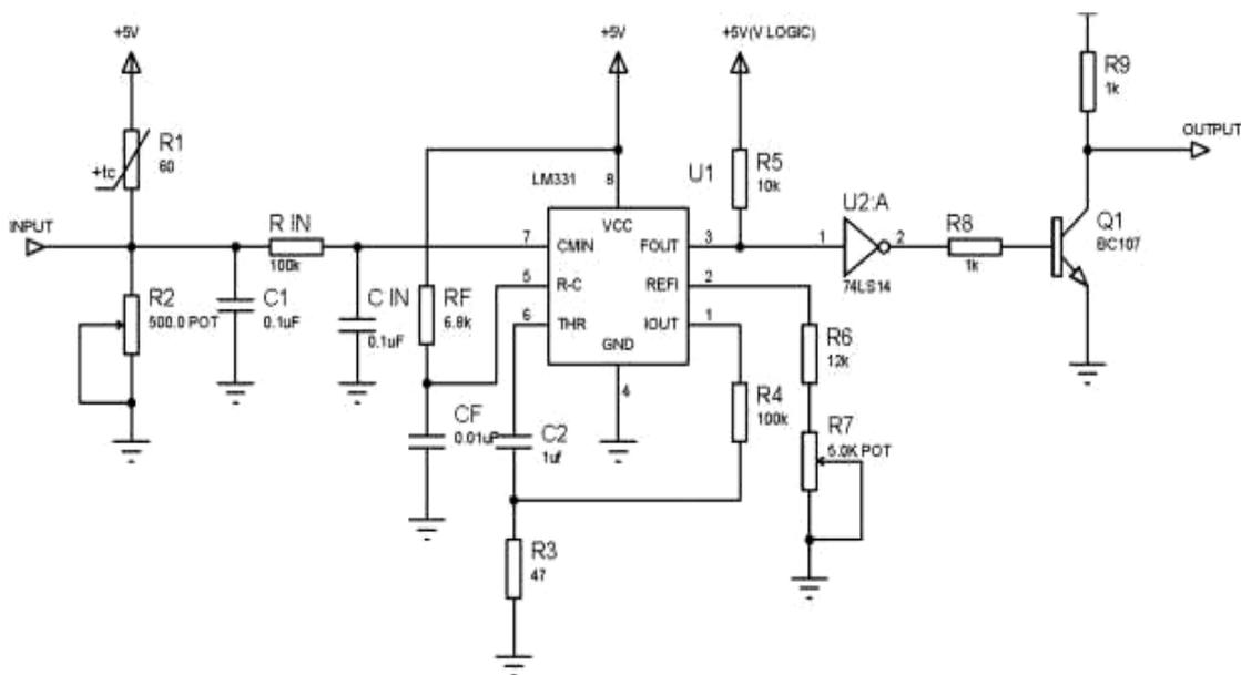
Fig. 3 (a). Transmitter circuit of measuring system.
