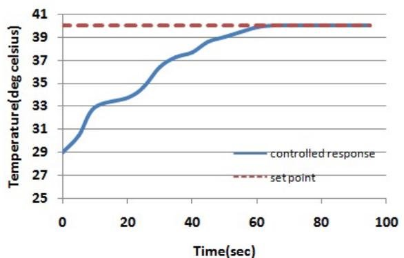
Fig. 6. Closed loop response of the system.
