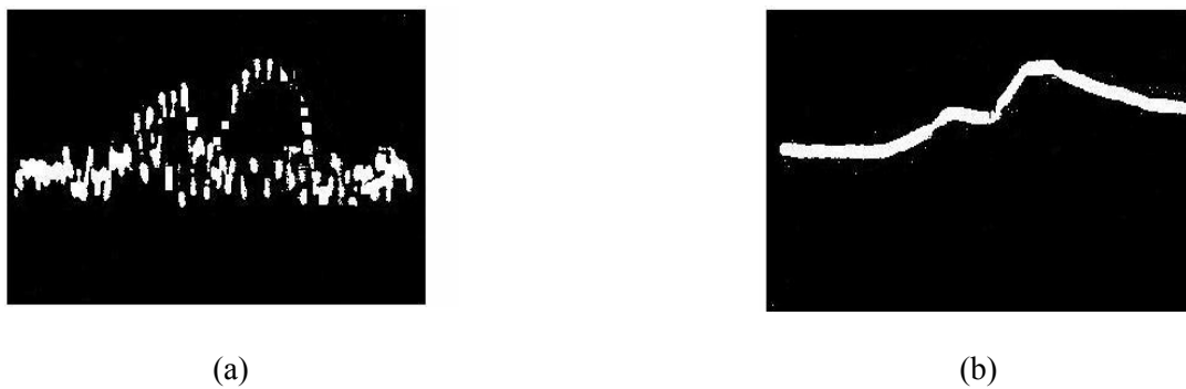
Fig. 7. The line scan of two holes before and after filtering.
