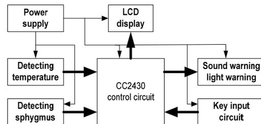
Fig. 1. The hardware diagram of the instrument.
