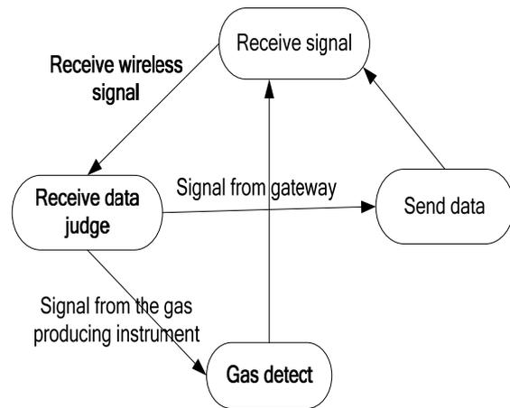
Fig. 10. The state diagram of detecting the poisonous gas state machine.
