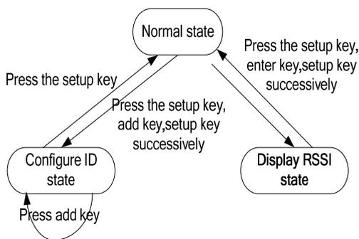
Fig. 9. The key state diagram.
