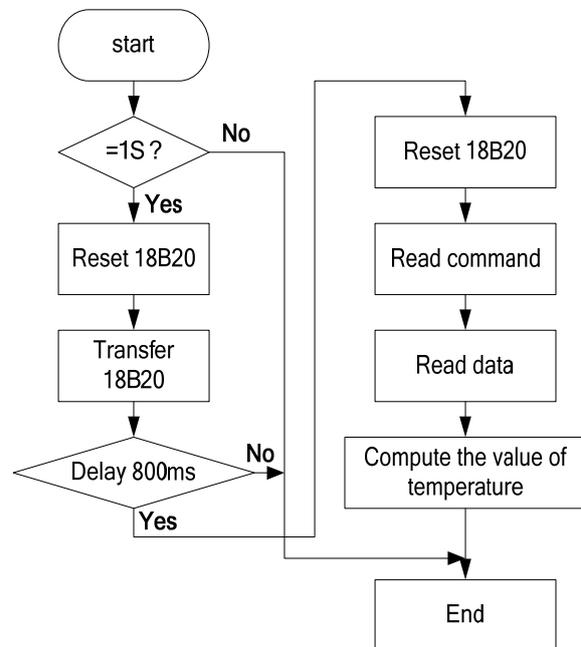
Fig. 8. The diagram of read temperature.
