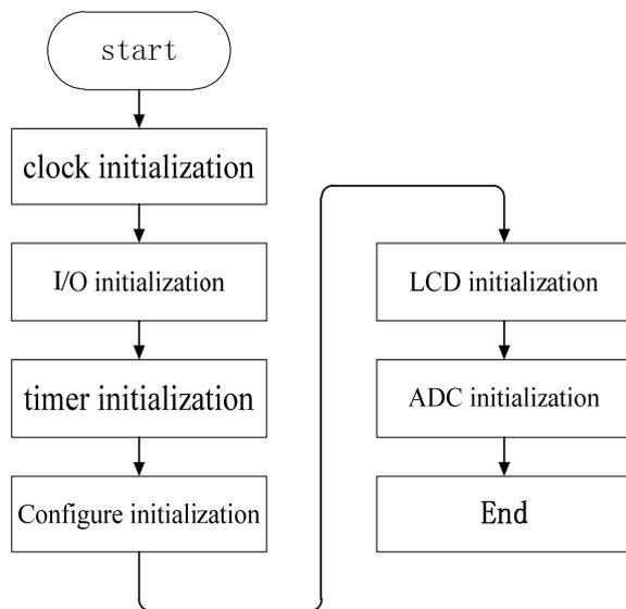
Fig. 6. The diagram of initialization.
