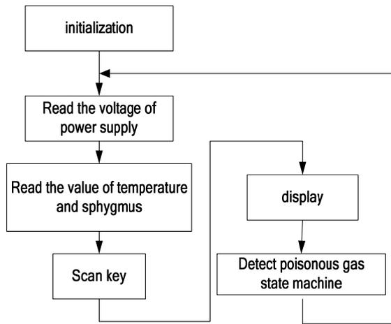
Fig. 5. The software diagram of the instrument.
