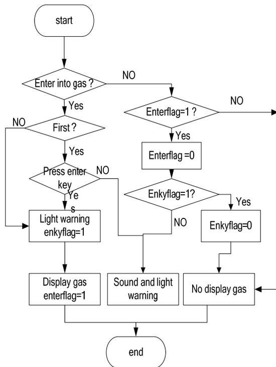
**Fig. 11.** The diagram of detecting the poisonous gas.**Table 2.** Format of message of instrument.
