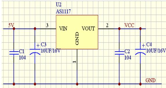
Fig. 2. The circuit of the power supply.
