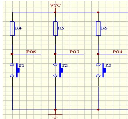
Fig. 4. The key circuit.
