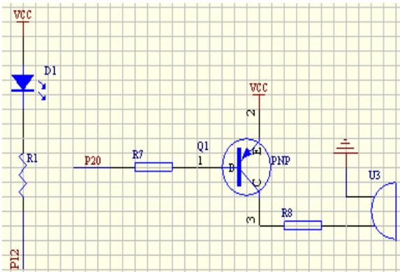
Fig. 3. Warning circuit.
