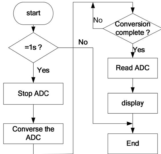
Fig. 7. The diagram of read the voltage of power supply
