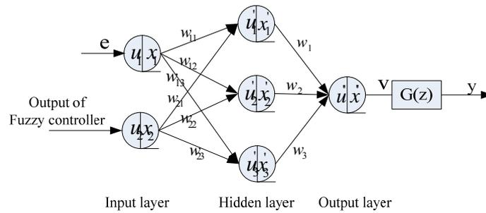
Fig. 2. PID neural network structure.
