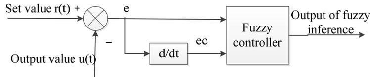
Fig. 1. Fuzzy PID controller structure diagram.
