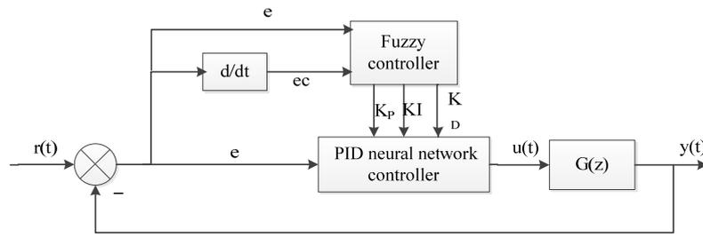
Fig. 3. Fuzzy Neural Network PID Controller schematic structure.
