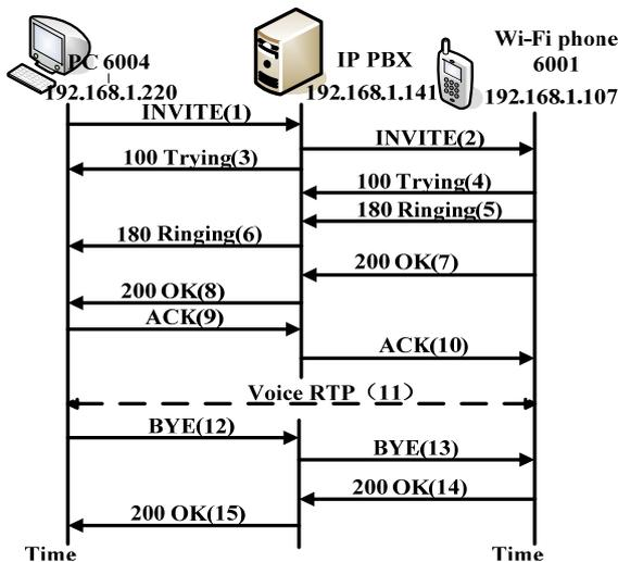
Fig. 12. Calling process of user through IP PBX.
