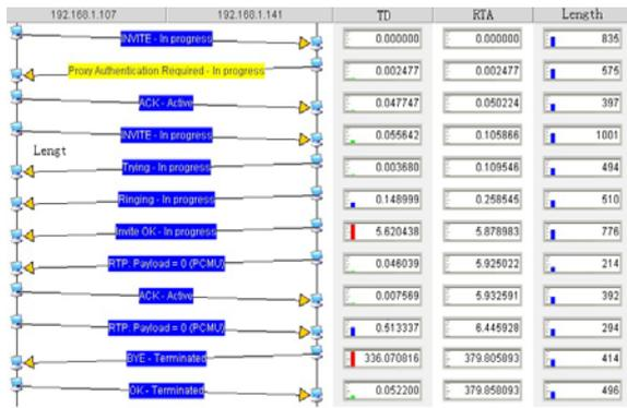
Fig. 9. The communication process chart between 6001 and IP PBX.
