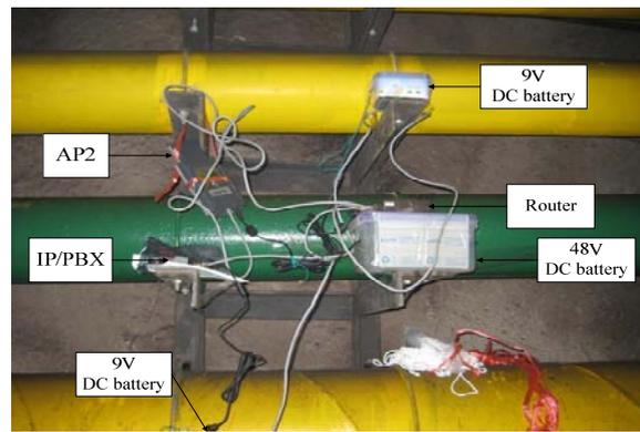
(b) Equipment connection of testing network
