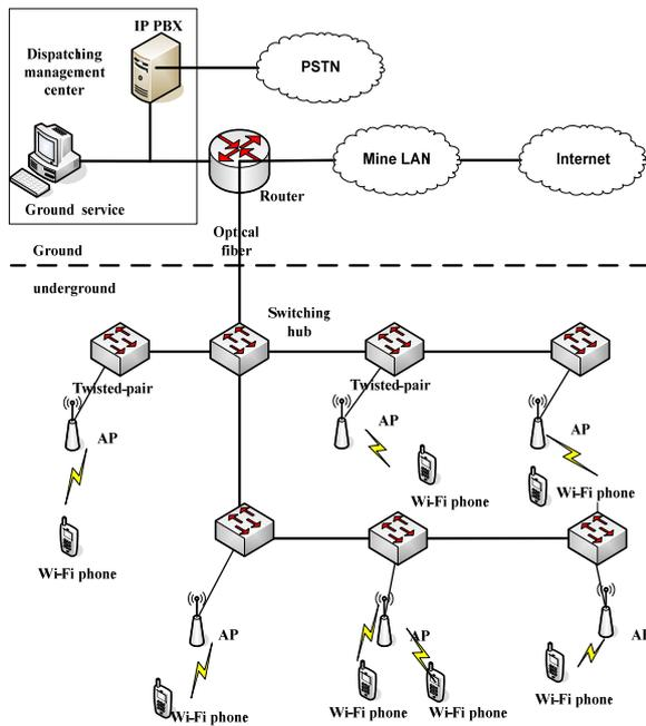
Fig. 1. Network topology of the wireless information system for underground coal mine.
