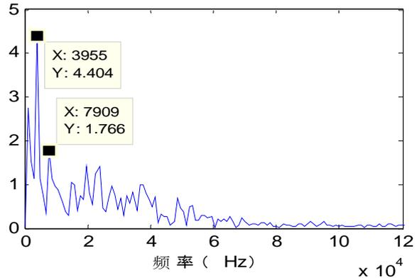
Fig. 15. Laplace wavelet correlation coefficient frequency (speed at 1500 rpm).
