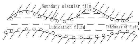
Fig. 2. Fluid friction.
