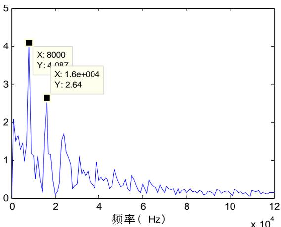
Fig. 14. Laplace wavelet correlation coefficient frequency spectrum (speed at 300 rpm).
