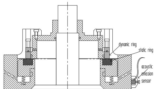
Fig. 7. Mechanical fluid seal structure.
