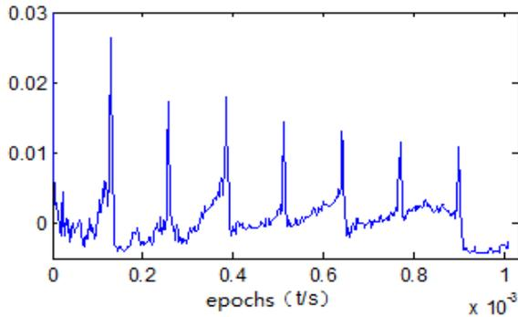
Fig. 12. Laplace wavelet filtering correlation coefficients.
