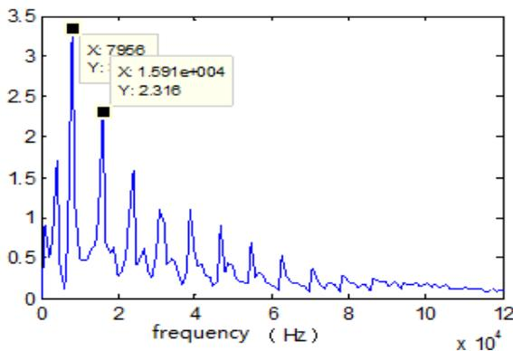
Fig. 13. Laplace wavelet correlation coefficient frequency spectrum (speed at 10 rpm).
