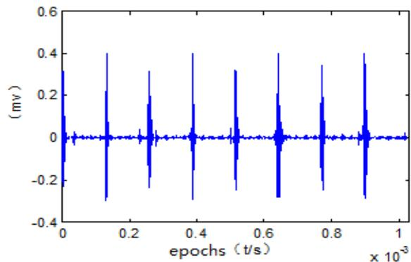
Fig. 11. AE signal time domain waveform after filtering.
