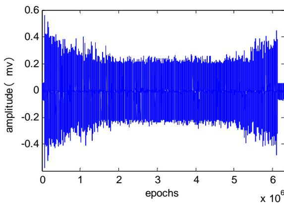
Fig. 4. Mechanical fluid seal end faces AE signal time domain waveform.
