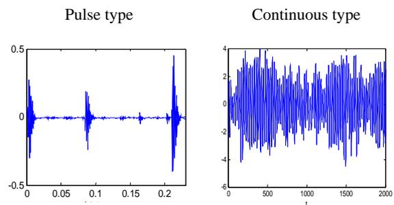
Fig. 5. Acoustic emission signal.
