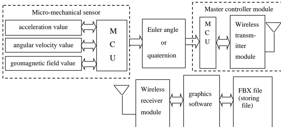
Fig. 2. System data flow and function of the inertial sensor.
