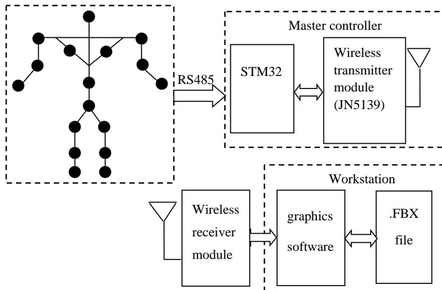
Fig. 6. Data transmission and hardware relationship of human MCS.
