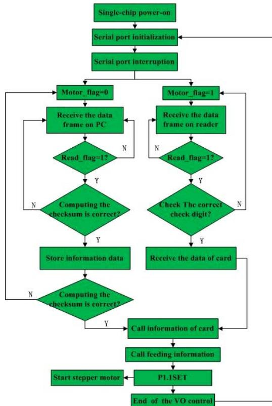
Fig. 6. Process diagram of MCU program.
