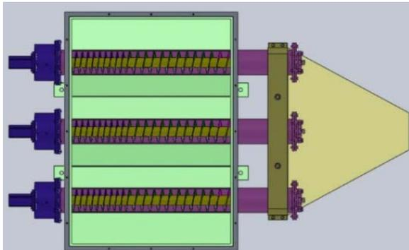
Fig. 3. Transporting device made by three sections of spiral.
