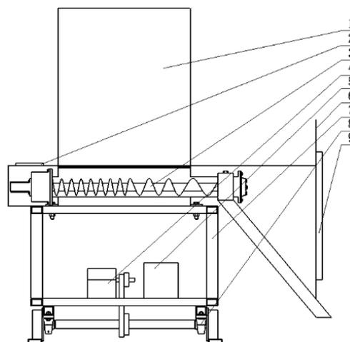
1 – Silo, 2 – Control systems, 3 – Feeding device, 4 – Power and Transmission, 5 – Power, 6 – Antenna Holder, 7 – Rack, 8 – Walking device, 9 – Identification system.
