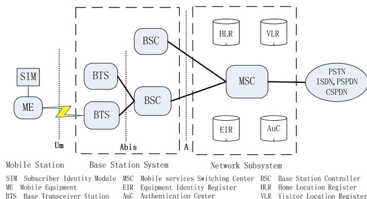
Fig. 1. The architecture of GSM communication network [5].
