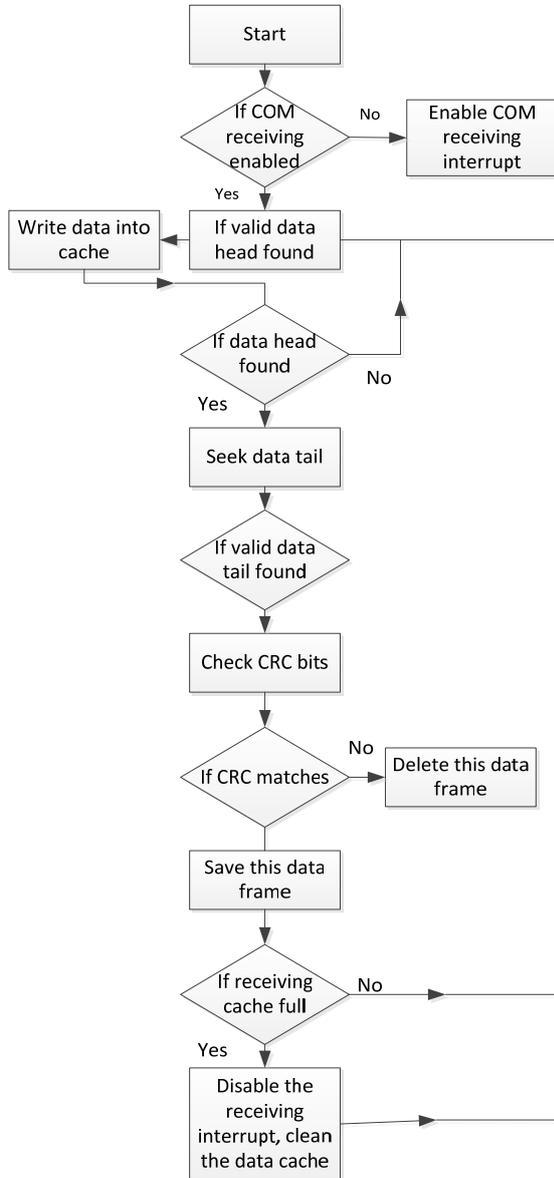
Fig. 11. The flow chart of coordinator processes the packages.
