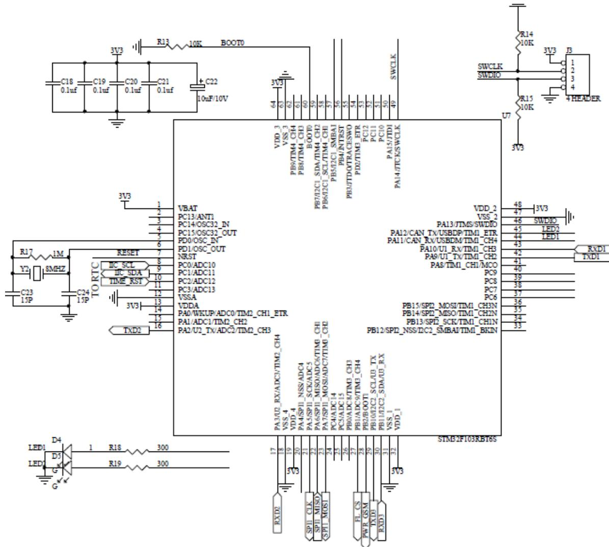
Fig. 3. The PCB of LQFP64 Pinout.
