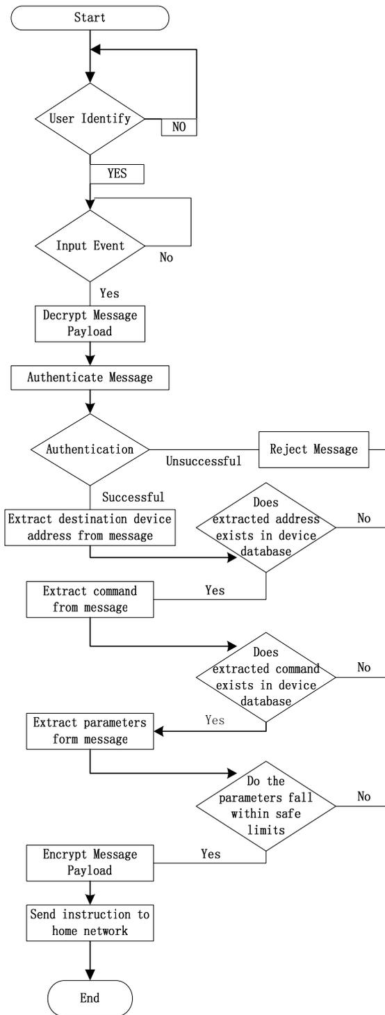
Fig. 12. The flow chart of the pre-processing system.
