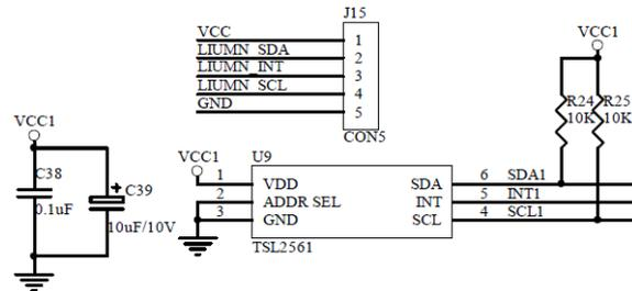
Fig. 5. The PCB of TSL2561 light sensor.
