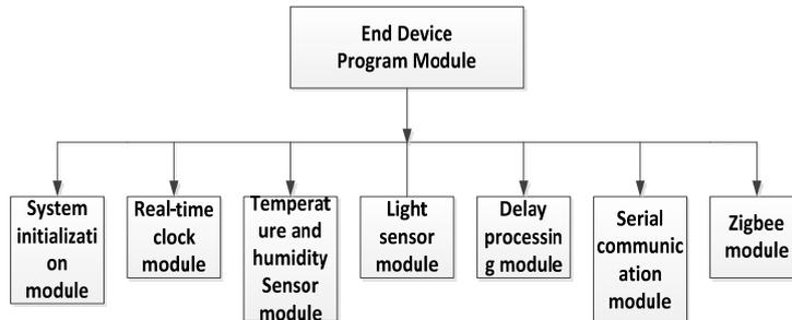
Fig. 8. The frame of end device program module.
