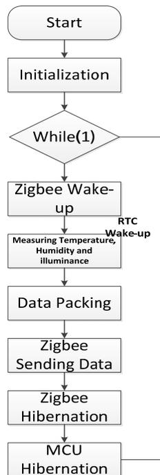
Fig. 9. The end device main program flow chart.
