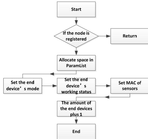
Fig. 10. The end device register flow chart.
