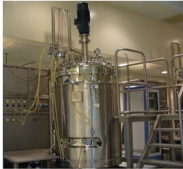
Fig. 1. WKT-30L fermentation experiment system.
