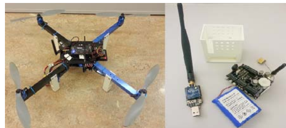
Fig. 3. (left) Drone assembled, embedding GPS and telemetry antenna. (right) Basestation node and wireless sensor node for pollution monitoring.
