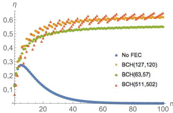
Fig. 2. Comparison of BCH codes.
