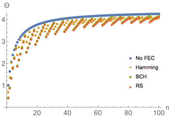
Fig. 11. Comparison of FEC codes at BER=4E-5.
