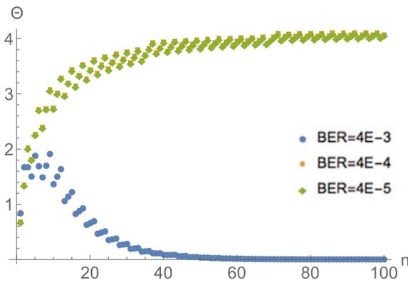
Fig. 6.  $\Theta$  for different BER values with Hamming code.
