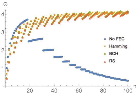
Fig. 10. Comparison of FEC codes at BER=4E-4.
