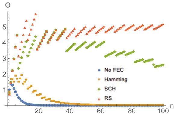
Fig. 9. Comparison of FEC codes at BER=4E-3.
