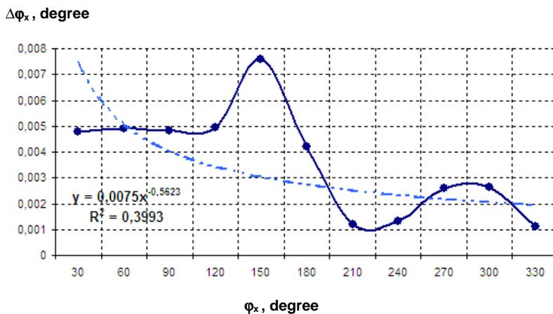
Fig. 5. Phase shift measurement absolute error (10 Hz, rectangular waveform input signals).
