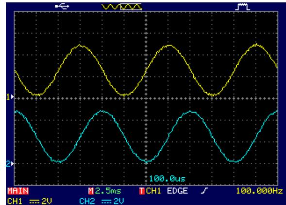
Fig. 4. Sine waveform input signals (90° phase shift, at 100 Hz).
