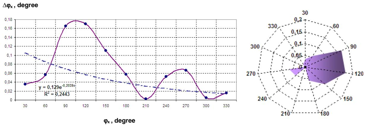
Fig. 9. Phase shift measurement absolute error (100 Hz, sine waveform input signals).
