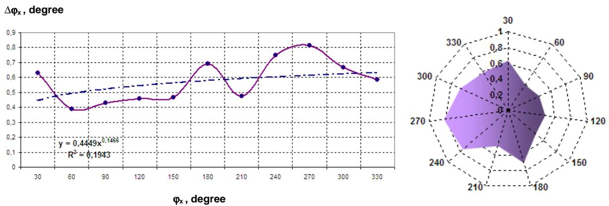
Fig. 10. Phase shift measurement absolute error (1 kHz, sine waveform input signals).
