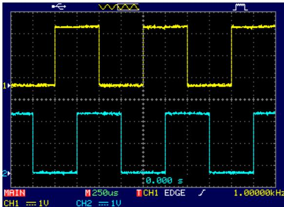
Fig. 3. Rectangular waveform input signals (120° phase shift, at 1 kHz).
