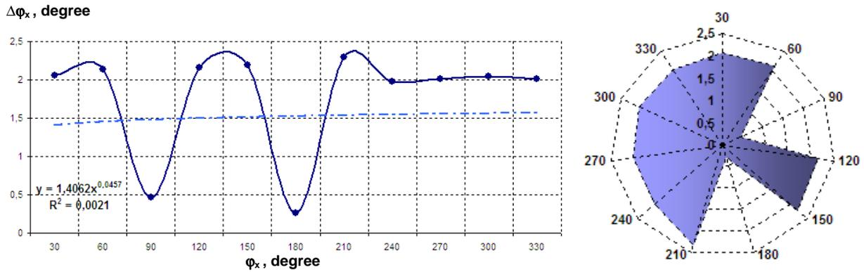
Fig. 8. Phase shift measurement absolute error (4 kHz, rectangular waveform input signals).
