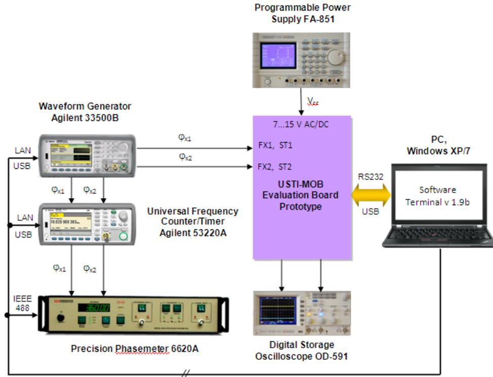
Fig. 1. Diagram of experimental measurement set-up for phase difference measurements.
