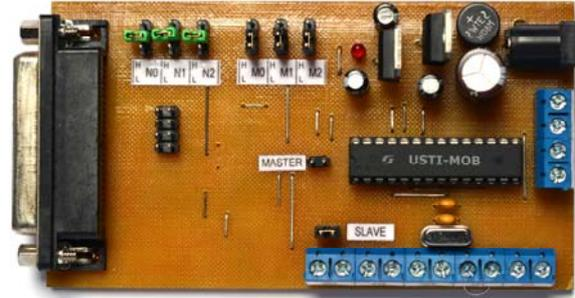
Fig. 1. Prototype of the USTI-MOB development board.
