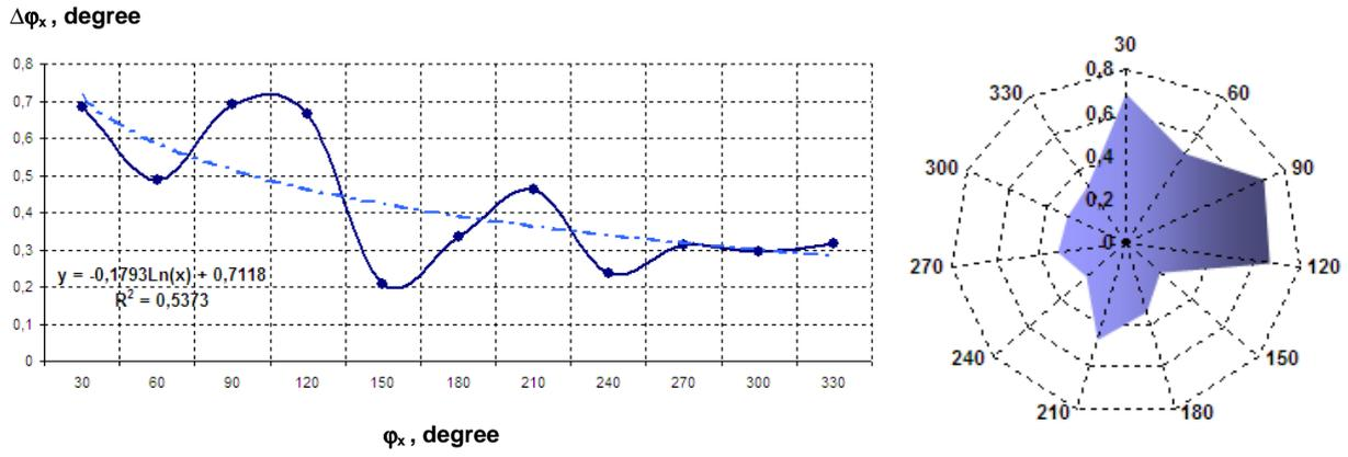
Fig. 7. Phase shift measurement absolute error (1 kHz, rectangular waveform input signals).
