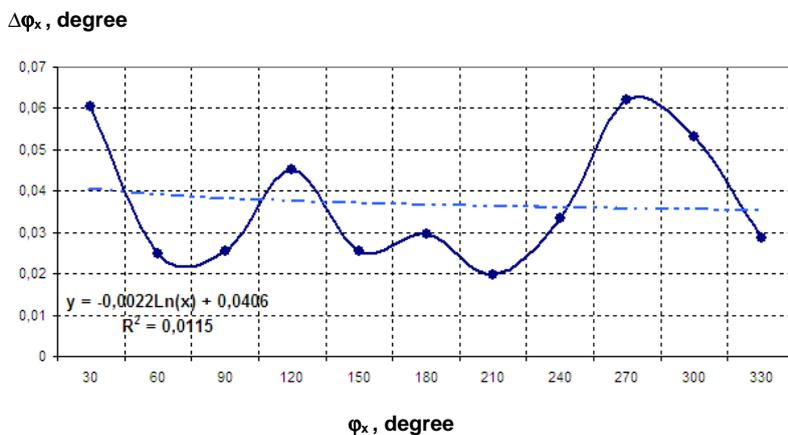
Fig. 6. Phase shift measurement absolute error (100 Hz, rectangular waveform input signals).
