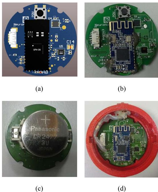
**Fig. 2.** (a) 3D version of the electronic circuit BLE-based temperature and humidity acquisition system; (b) Prototype board: Top view temperature and humidity sensor, microcontroller and BLE module; (c) Bottom view of the device; (d) Top view of prototype board with a CR2477 Panasonic battery inside plastic box.
