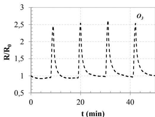
**Fig. 5.** Normalized response of the ozone sensor based on ZnO nanoparticles deposited by nozzle-less spray under 500 ppb  $O_3$  at 200 °C.
