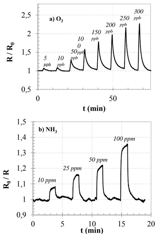
**Fig. 7.** Response of the flexible gas sensor based on ZnO nanoparticles deposited by nozzle-less spray over different gas concentrations: a)  $O_3$  from 5 ppb to 300 ppb at 200 °C, and b)  $NH_3$  from 10 ppm to 100 ppm at 300 °C.
